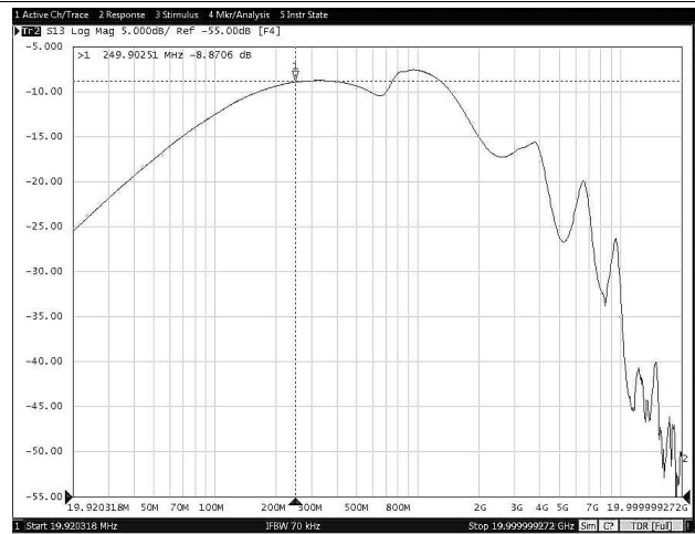
图 32. Off-State Data-Switch Isolation vs Frequency (TPS25830-Q1)
