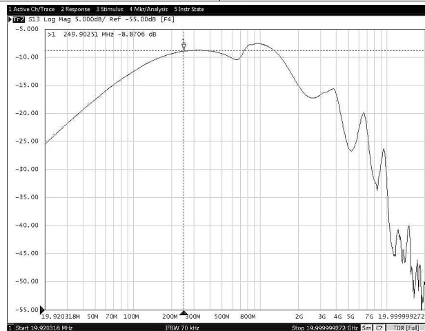
图 31. Data Transmission Characteristics vs Frequency (TPS25830-Q1)
