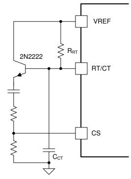
Figure 28. Current Mode PWM Used as a Voltage Mode PWM
