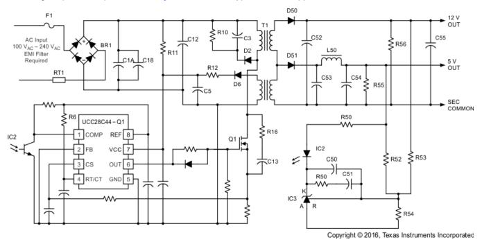
Figure 29. Typical Off-Line Application
