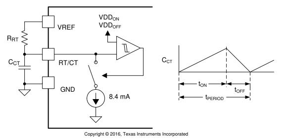
Figure 23. Oscillator Circuit
