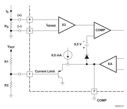
$I_{S} = \frac{\left(\text{R2} \times \frac{\text{V}_{REF}}{\text{R1} + \text{R2}}\right) - 0.5}{3\text{R}_{S}}$  NOTE: Peak current (I<sub>S</sub>) is determined by the formula:
