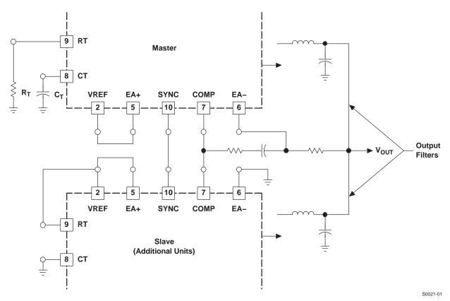
NOTE: Slaving allows parallel operation of two or more units with equal current sharing.
