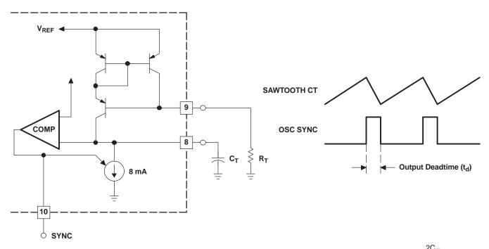
NOTE: Output deadtime is determined by the size of the external capacitor,  $C_T$ , according to the formula: For large values of  $R_T$ :  $Td = 250 \ C_T$
