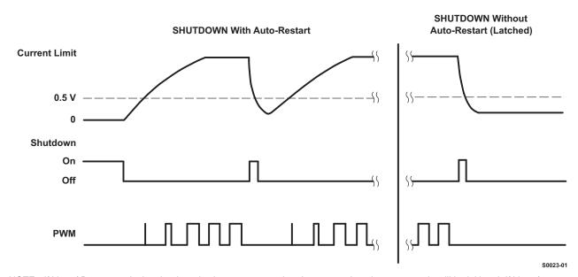
NOTE: If  $V_{REF}$  / R1 < 0.8 mA, the shutdown latch commutates when  $I_{SS}$  = 0.8 mA and a restart cycle will be initiated. If  $V_{REF}$  / R1 > 3 mA, the device will latch off until power is recycled.
