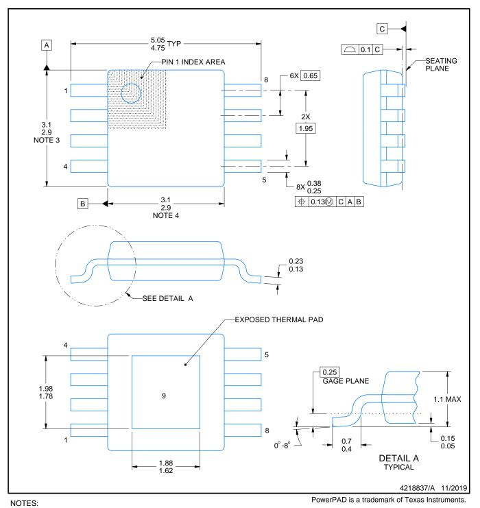
1. All linear dimensions are in millimeters. Any dimensions in parenthesis are for reference only. Dimensioning and tolerancing per ASME Y14.5M. 2. This drawing is subject to change without notice. 3. This dimension does not include mold flash, protrusions, or gate burrs. Mold flash, protrusions, or gate burrs shall not
