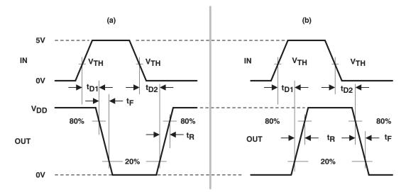
The 20% and 80% thresholds depict the dynamics of the bipolar output devices that dominate the power MOSFET transition through the Miller regions of operation.
