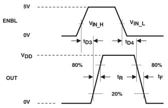
The 20% and 80% thresholds depict the dynamics of the bipolar output devices that dominate the power MOSFET transition through the Miller regions of operation.
