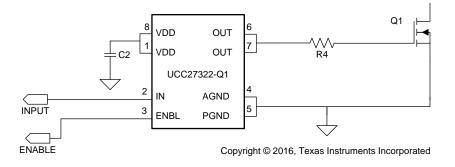
Figure 27. Typical Application Diagram of UCC27322-Q1
