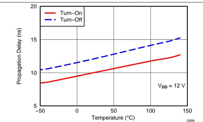
图 14. Input To Output Propagation Delay vs Temperature
