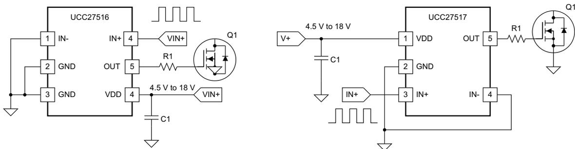
(IN- Is Grounded to the Enable Output)
