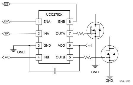
Figure 29. UCC2752x Typical Application Diagram (X = 8)
