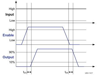
Figure 1. Enable Function (For Non-Inverting Input Driver Operation)
