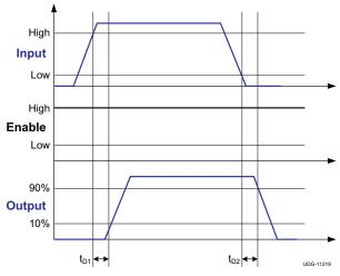
Figure 3. Non-Inverting Input Driver Operation
