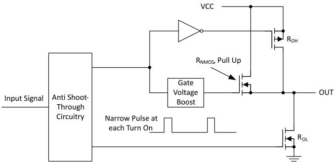
Figure 27. UCC2752x Gate Driver Output Structure
