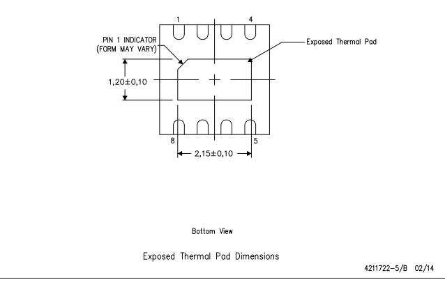
NOTE: A. All linear dimensions are in millimeters
