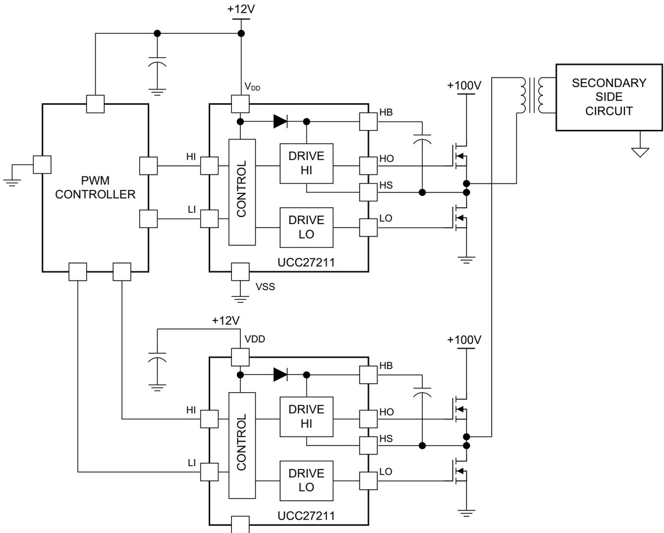
**Figure 19. UCC27211 Typical Application Diagram**
