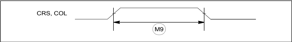
Figure 38. MII async inputs timing diagram
