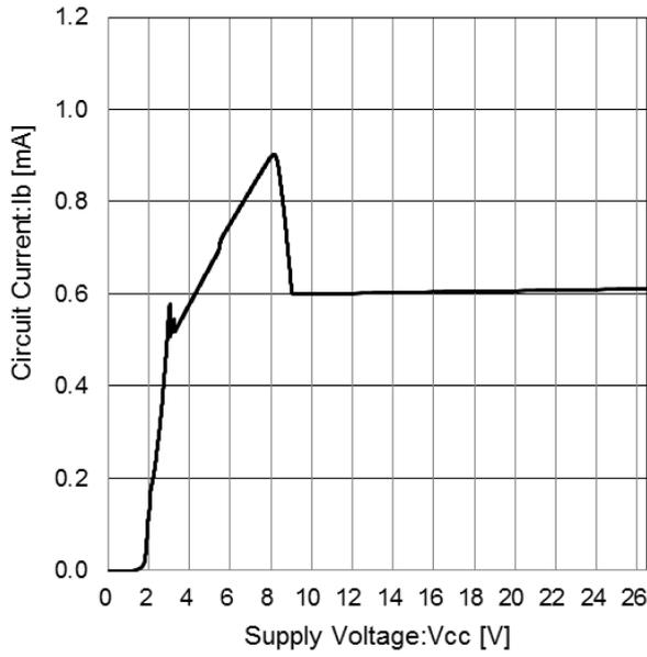
Figure 13. Circuit Current
