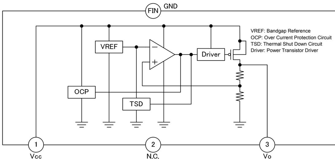
Figure 3. Block Diagram
