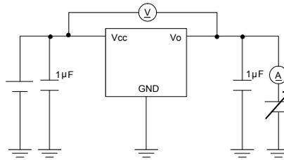
Measurement Circuit of Figure 8 and Figure 17
