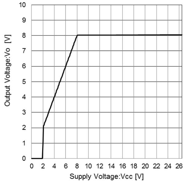
Figure 5. Line Regulation ( $I_o=0\text{mA}$ )
