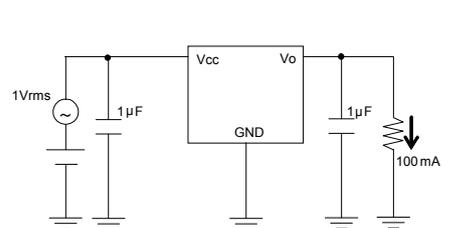
Measurement Circuit of Figure 9 and Figure 18
