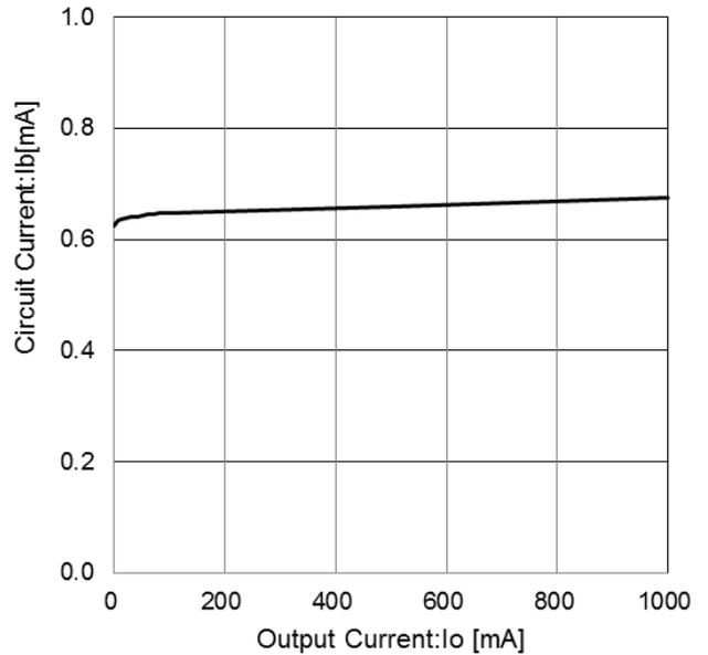
Figure 11. Circuit Current
