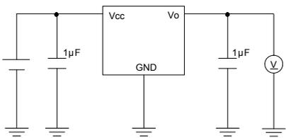
Measurement Circuit of Figure 10 and Figure 19
