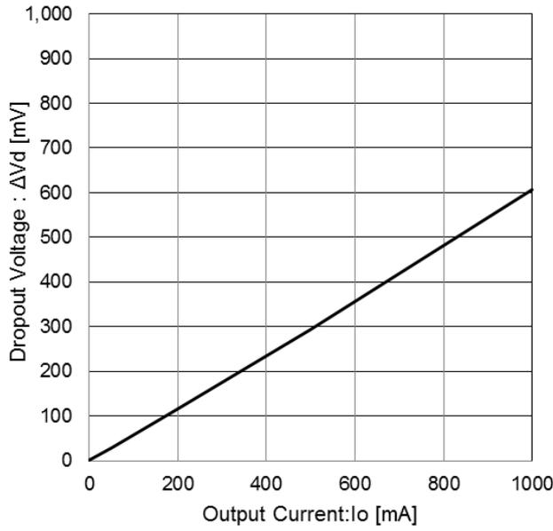
Figure 17. Dropout Voltage
