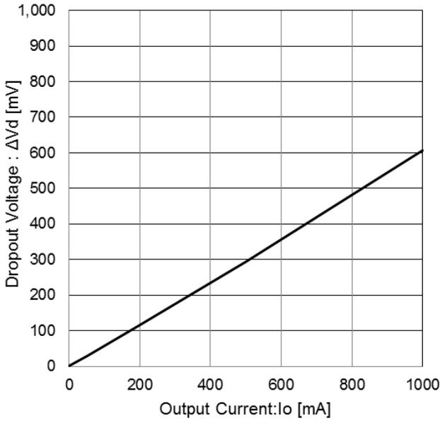
Figure 8. Dropout Voltage
