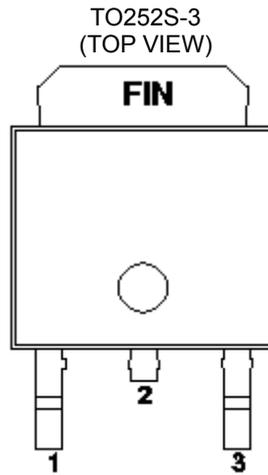
Figure 2. Pin Configuration
