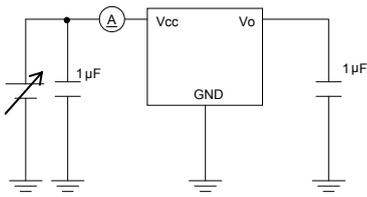
Measurement Circuit of Figure 4 and Figure 13
