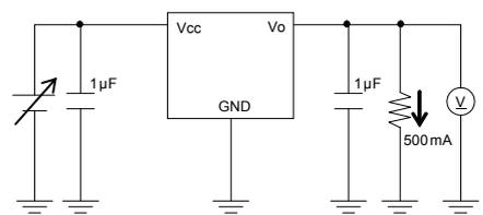
Measurement Circuit of Figure 6 and Figure 15
