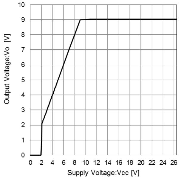
Figure 14. Line Regulation (Io=0mA)
