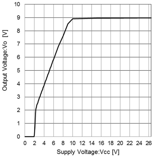
Figure 15. Line Regulation (Io=500mA)
