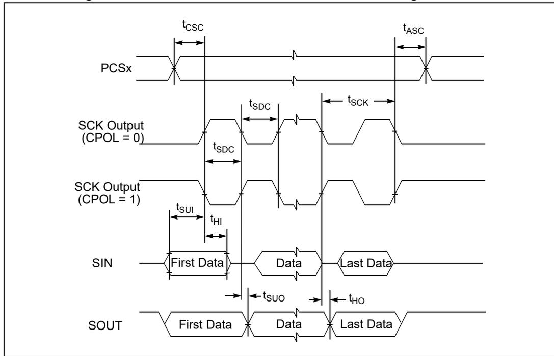
Figure 22. DSPI CMOS master mode — classic timing, CPHA = 1
