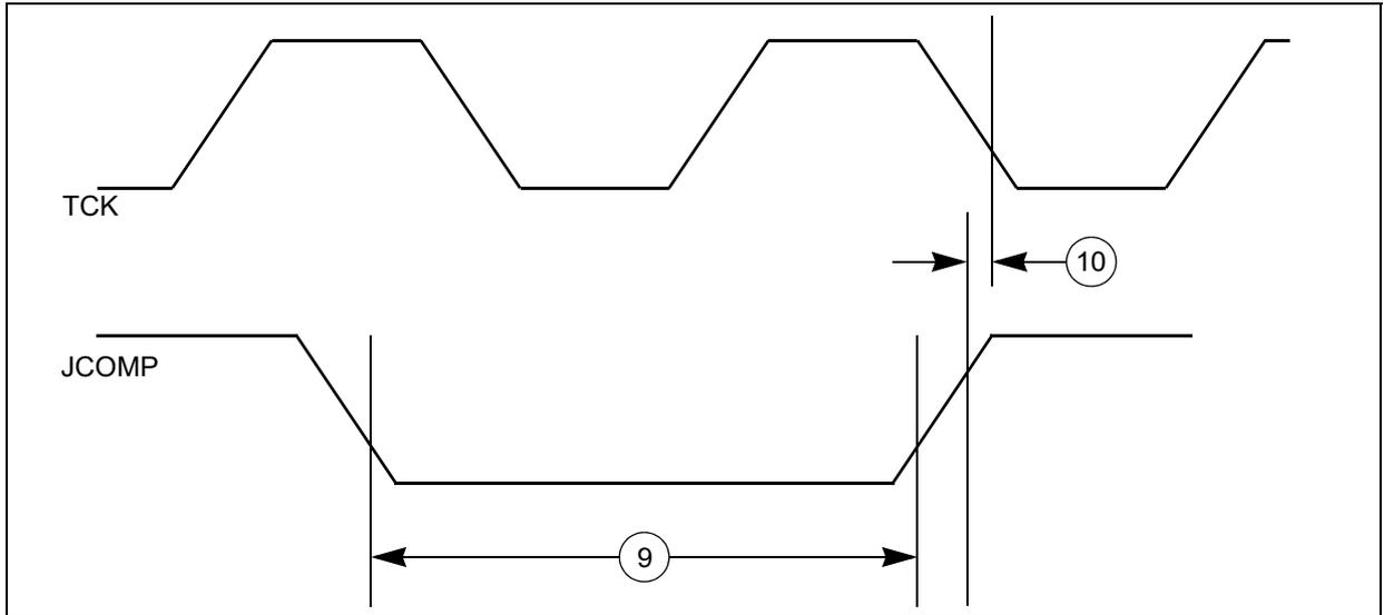
Figure 15. JTAG boundary scan timing
