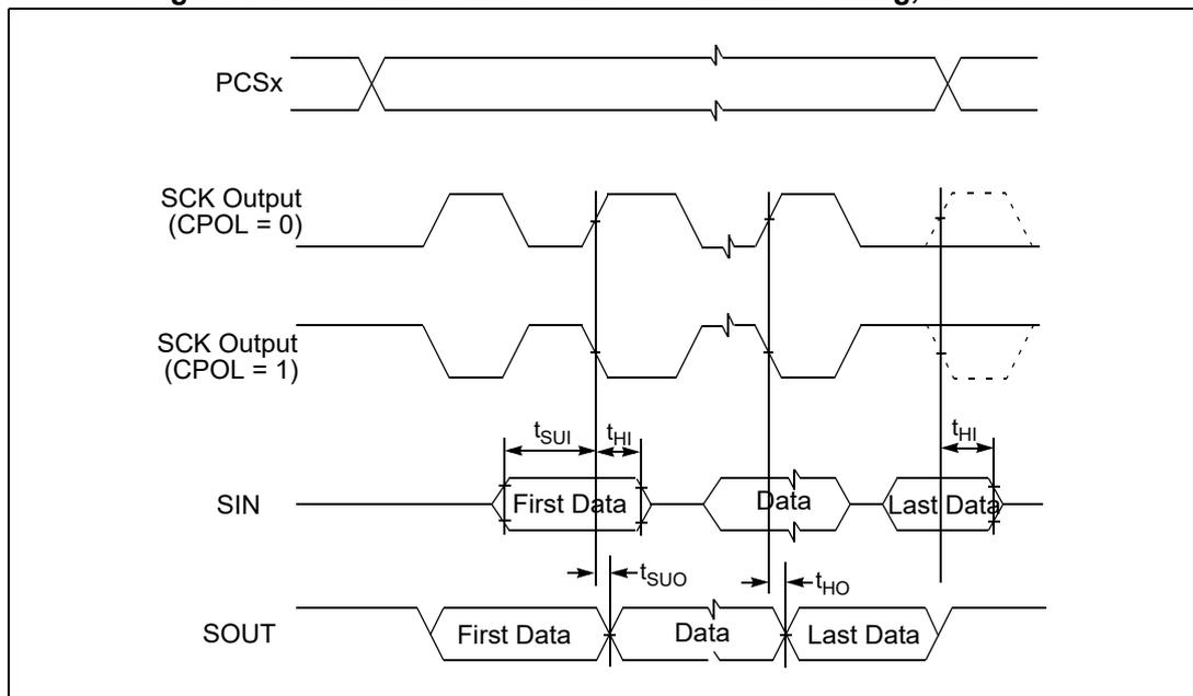
Figure 26. DSPI PCS strobe ( $\overline{\text{PCSS}}$ ) timing (master mode)
