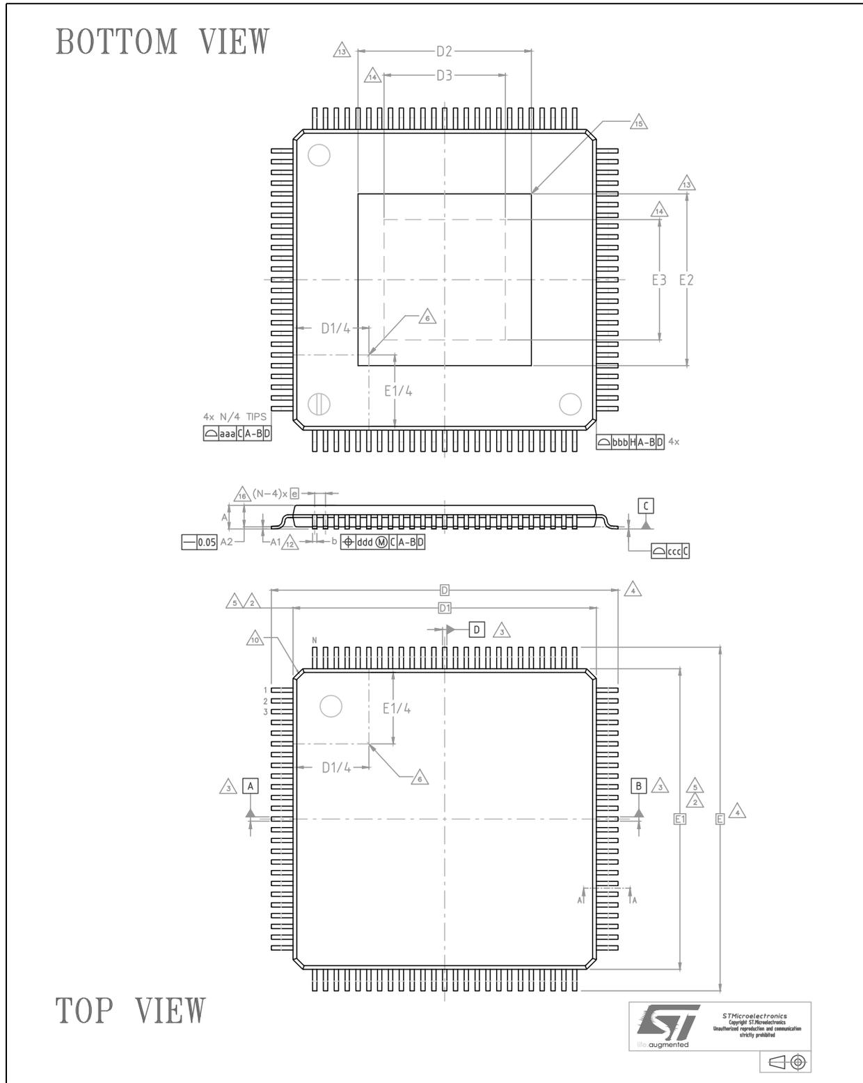
Figure 35. eTQFP100 section A-A
