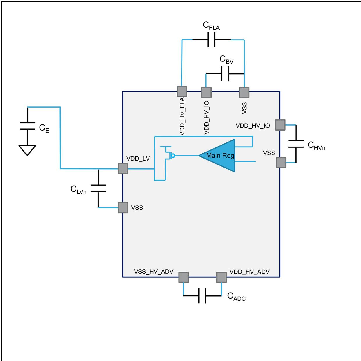
Figure 10. Standby regulator with internal ballast mode
