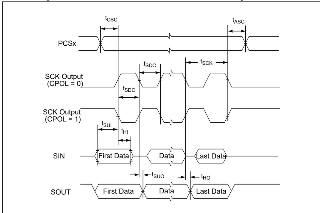
**Figure 25. DSPI CMOS master mode — modified timing, CPHA = 1**
