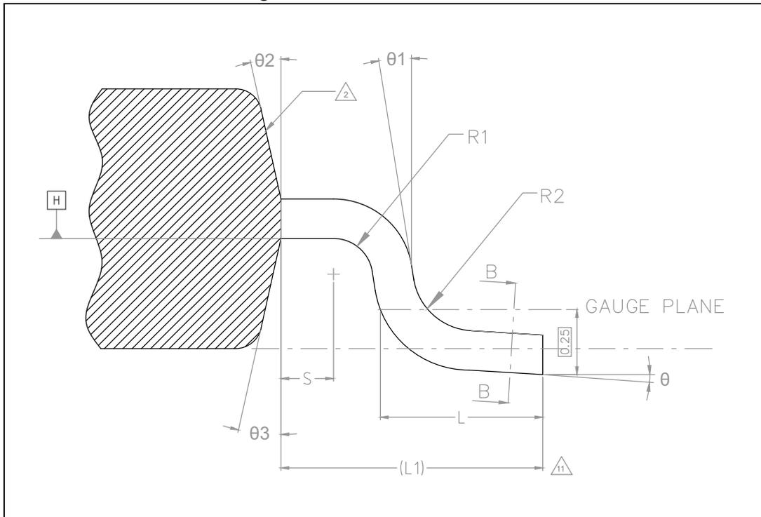
Figure 32. eTQFP64 section B-B
