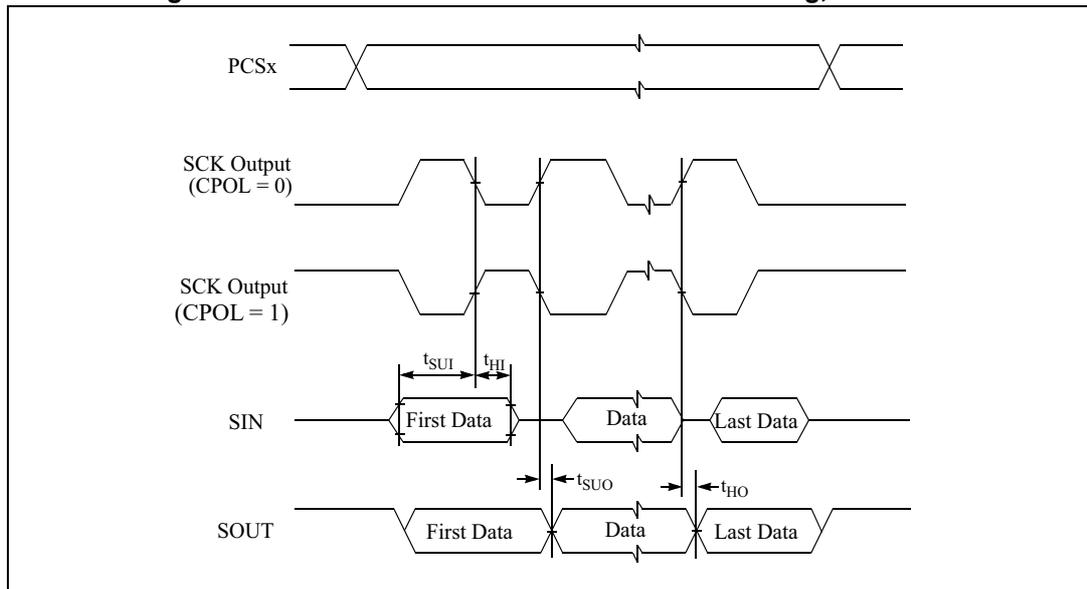
Figure 23. DSPI PCS strobe (PCSS) timing (master mode)
