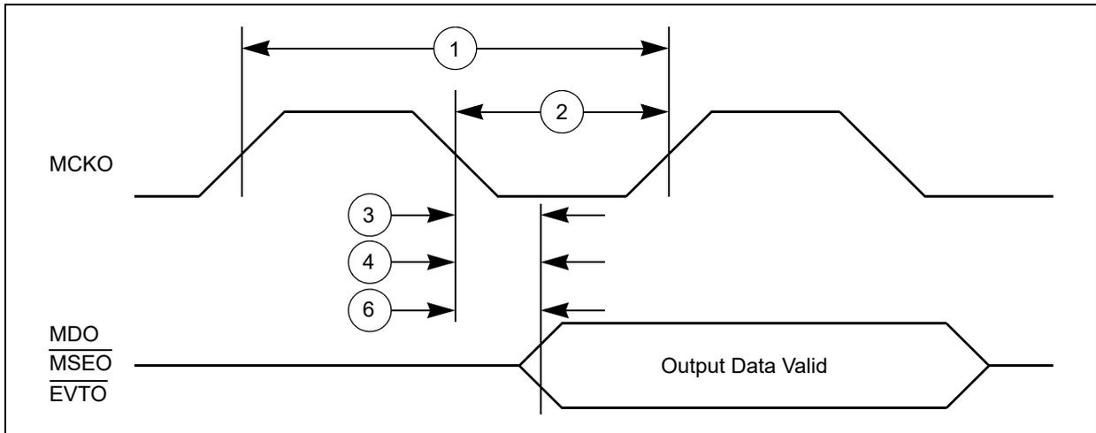
Figure 17. Nexus event trigger and test clock timings
