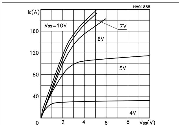
Figure 4. Transfer characteristics
