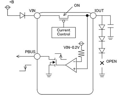
Figure 18. LED Open detection function
