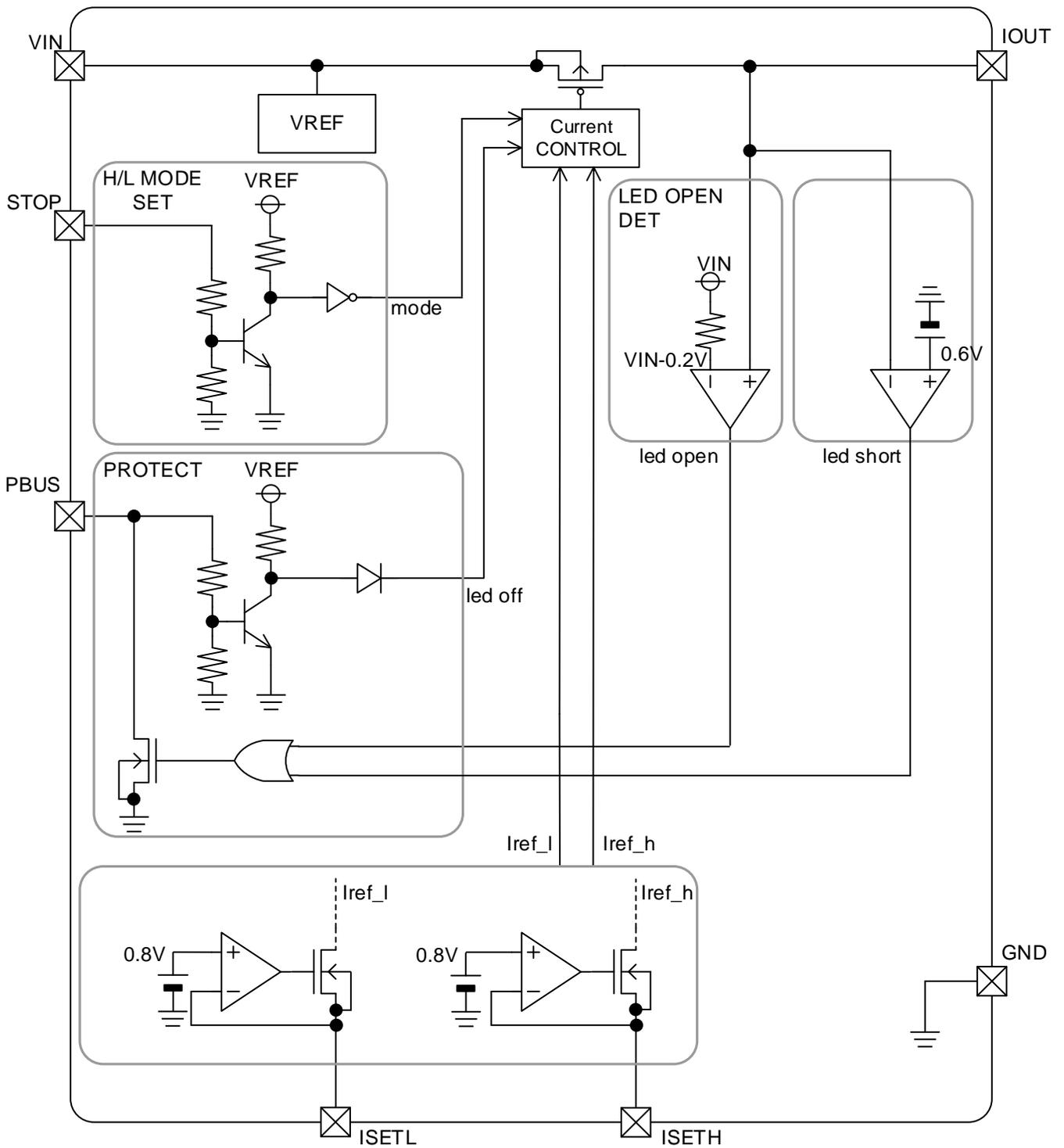
Figure 4. Block Diagram
