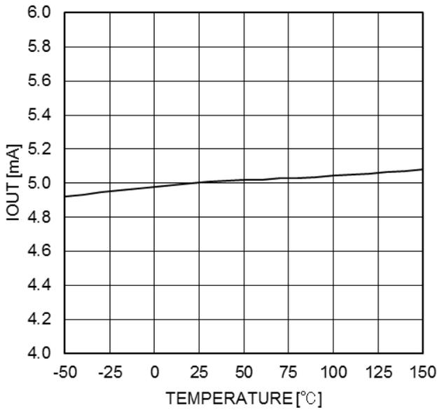
Figure 9.  $I_{OUT}$  vs  $T_a$
