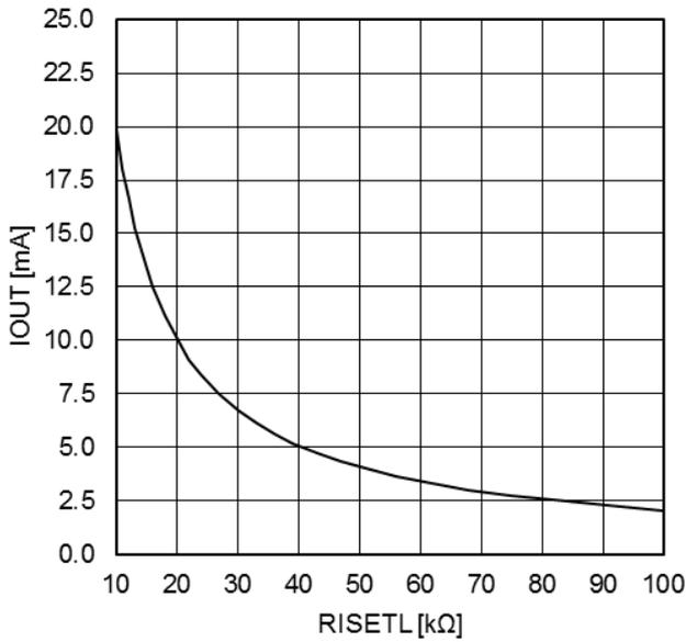
Figure 5.  $I_{OUT}$  vs  $R_{ISETL}$  (STOP=Low)
