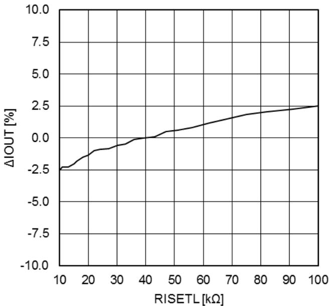
Figure 11.  $\Delta I_{OUT}$  vs  $R_{ISETL}$
