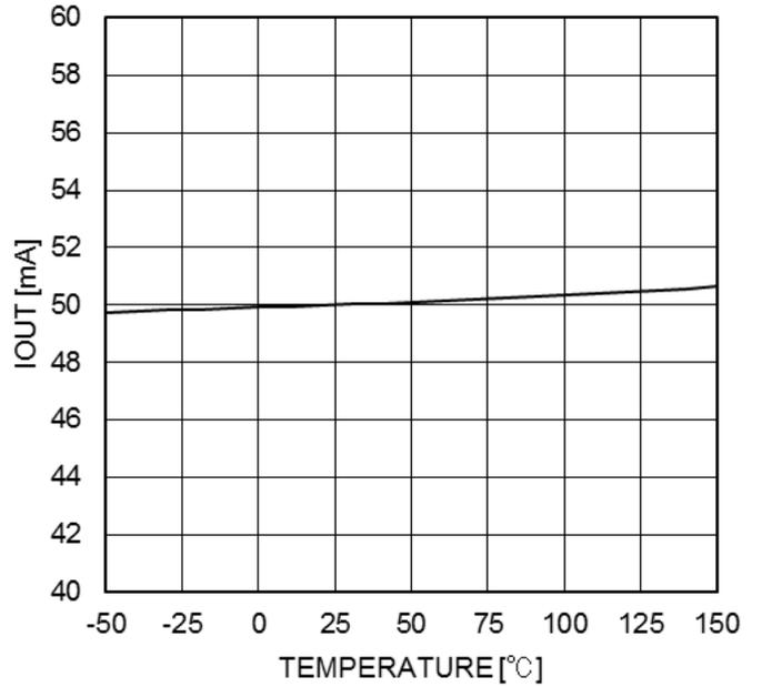
Figure 10.  $I_{OUT}$  vs  $T_a$
