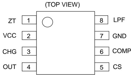
Figure 2. Pin Configuration
