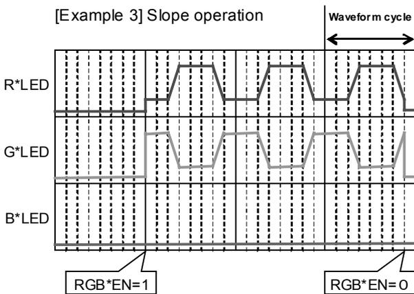
When a rising/falling slope time is longer than the setting made in example 2, a continuous color change is made by slope operation.
