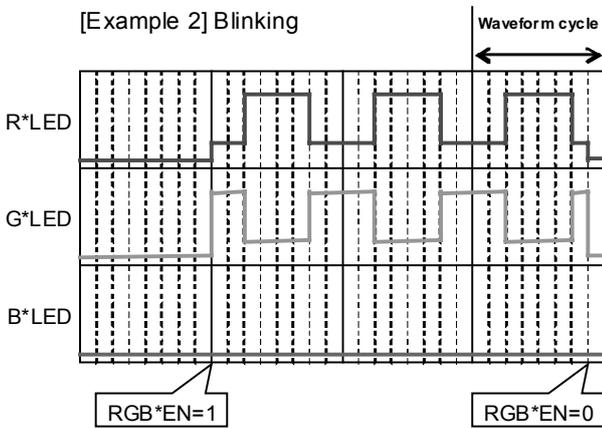
Setting a rising/falling slope time to "0" causes blinking to take place. Phase switching takes place via the setting currents of R and G.
