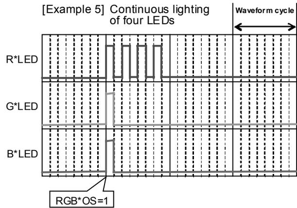
This example shows that lighting occurs continuously in the order of white, red, red and red. To achieve this, waveform patterns 16, 1 and RGB\*OS single cycle operation need to be combined.
