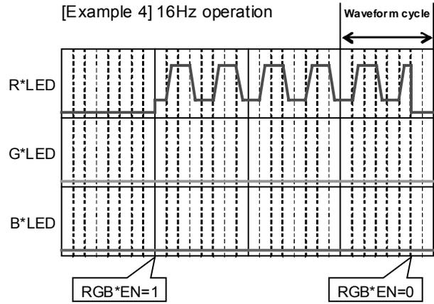
Combining the settings of a waveform pattern 11 and a waveform cycle 131ms causes blinking at a rate of 15.3Hz (approx. 16Hz).
