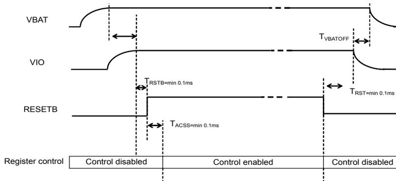
Figure 18. Power supply ON/OFF sequence
