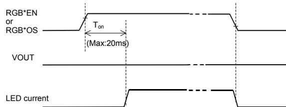
Figure 8. LED electric current When DC/DC isn't used.
