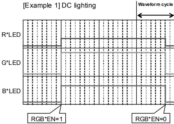
Selecting a waveform pattern 8 causes a continuous normal operation to take place through the setting current 1.
