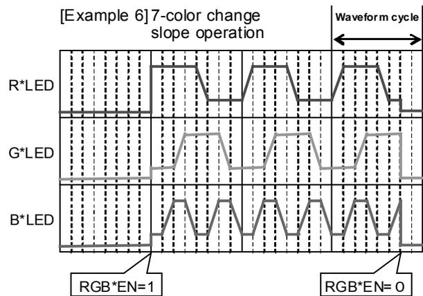
R, G and B waveform patterns are set in a way that any of R, G and B changes constantly.
