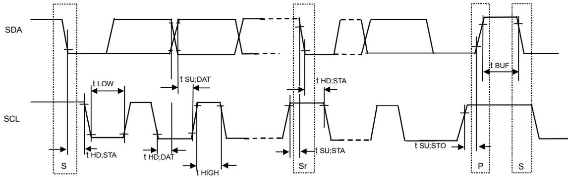
Figure 1 Timing diagram
