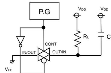
Figure 6. Propagation Delay Time CONT→OUT (tPZL, tPLZ) Test Circuit
