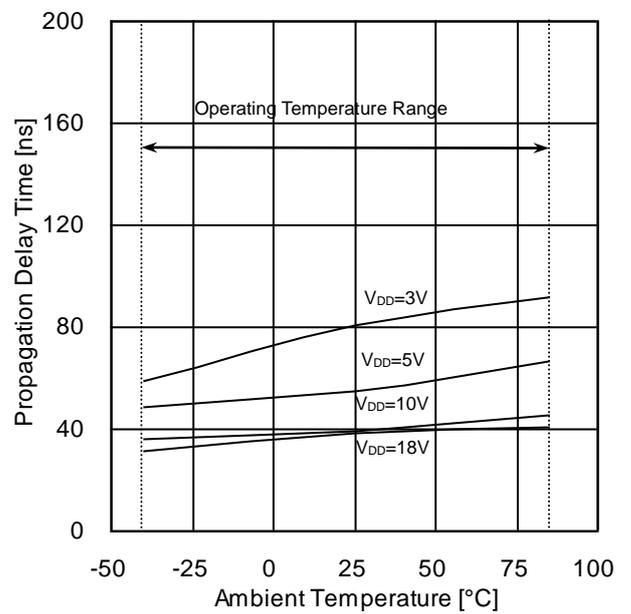
Figure 15. Propagation Delay Time CONT→OUT(t<sub>PHZ</sub>) vs Ambient Temperature
