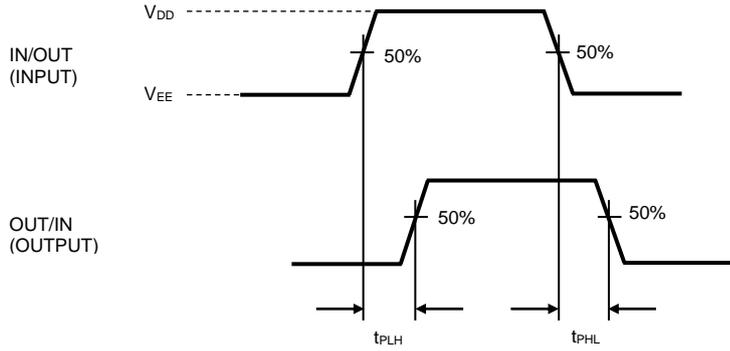
Figure 1. Propagation Delay Time IN→OUT (tPHZ, tPLZ) Input/Output Waveform
