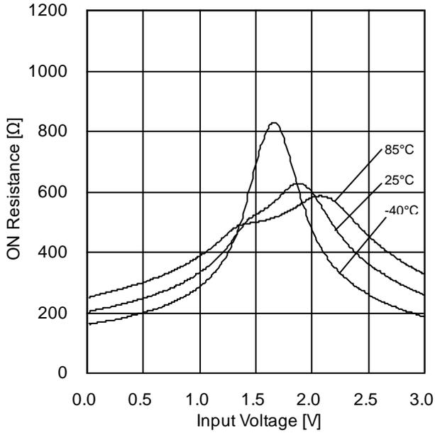
Figure 8. ON Resistance vs Input Voltage (V<sub>DD</sub>=3V, V<sub>EE</sub>=0V, CONT=3V)
