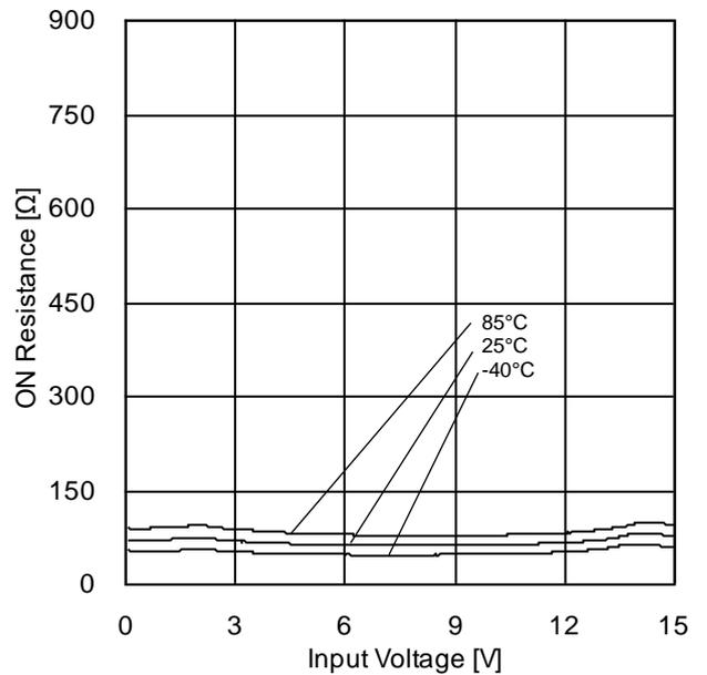
Figure 11. ON Resistance vs Input Voltage (V<sub>DD</sub>=15V, V<sub>EE</sub>=0V, CONT=15V)
