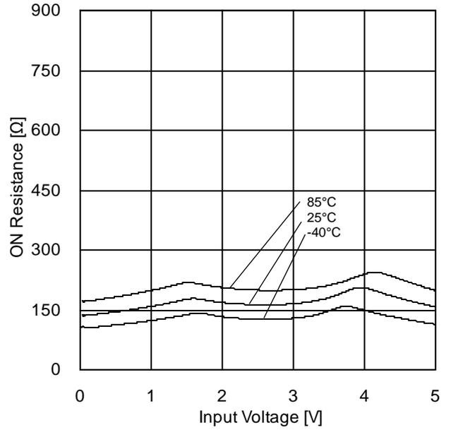
Figure 9. ON Resistance vs Input Voltage (V<sub>DD</sub>=5V, V<sub>EE</sub>=0V, CONT=5V)
