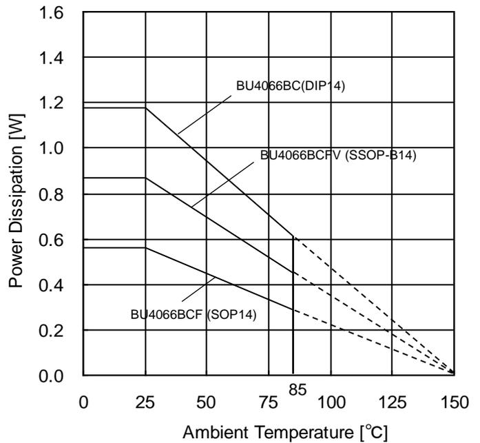
Figure 19. Derating Curve
