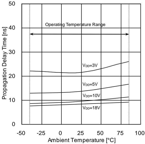
Figure 12. Propagation Delay Time IN→OUT(t<sub>PLH</sub>) vs Ambient Temperature
