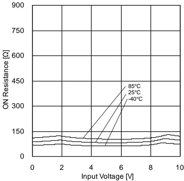
Figure 10. ON Resistance vs Input Voltage (V<sub>DD</sub>=10V, V<sub>EE</sub>=0V, CONT=10V)
