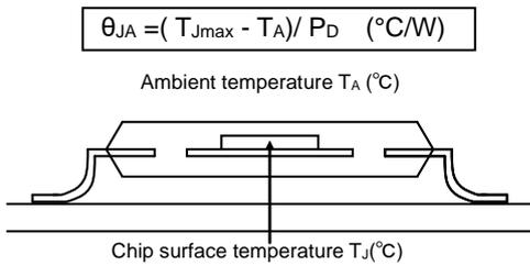
Figure 18. Thermal Resistance
