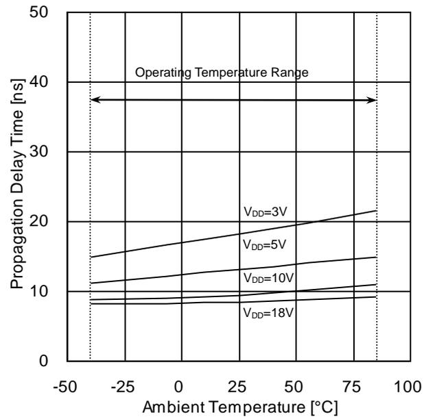
Figure 13. Propagation Delay Time IN→OUT(t<sub>PHL</sub>) vs Ambient Temperature
