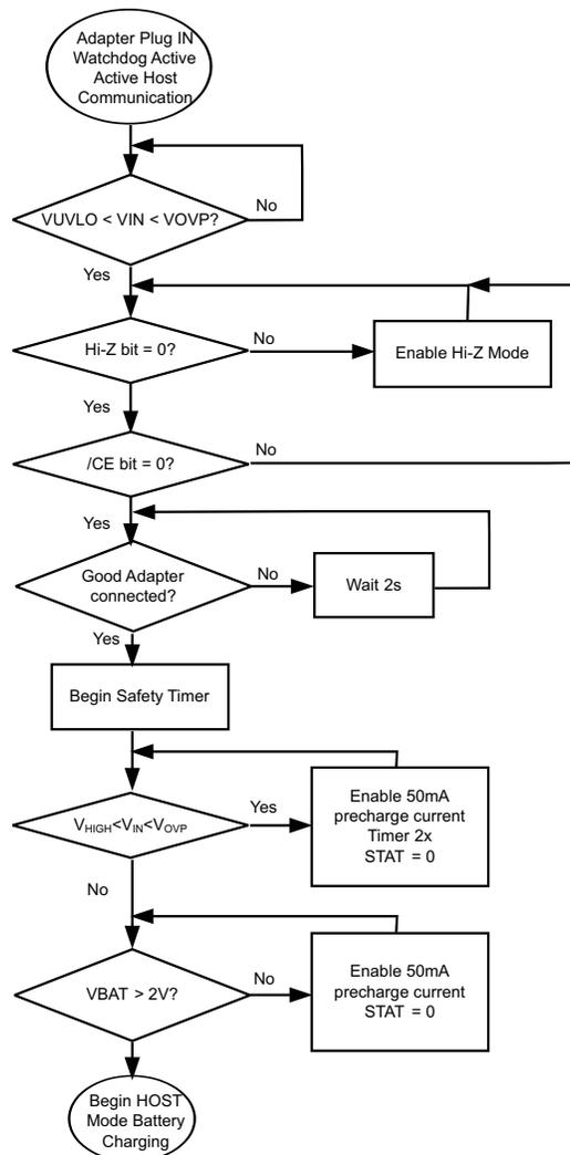
**Figure 27. Startup on Adapter Plug-In in Host-Controlled Mode**
