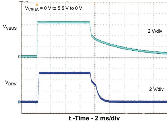
Figure 22. DRV Startup/Shutdown
