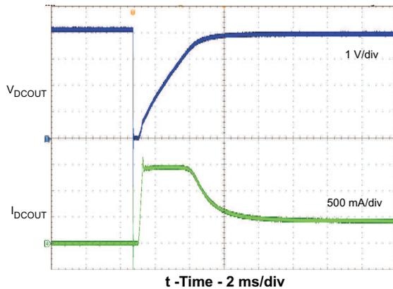
Figure 18. Hotplug 1000 $\mu F$  Capacitor into DCOUT
