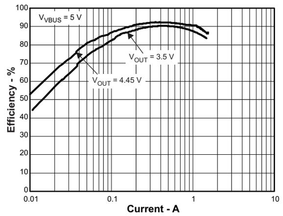
Figure 25. Charger Efficiency
