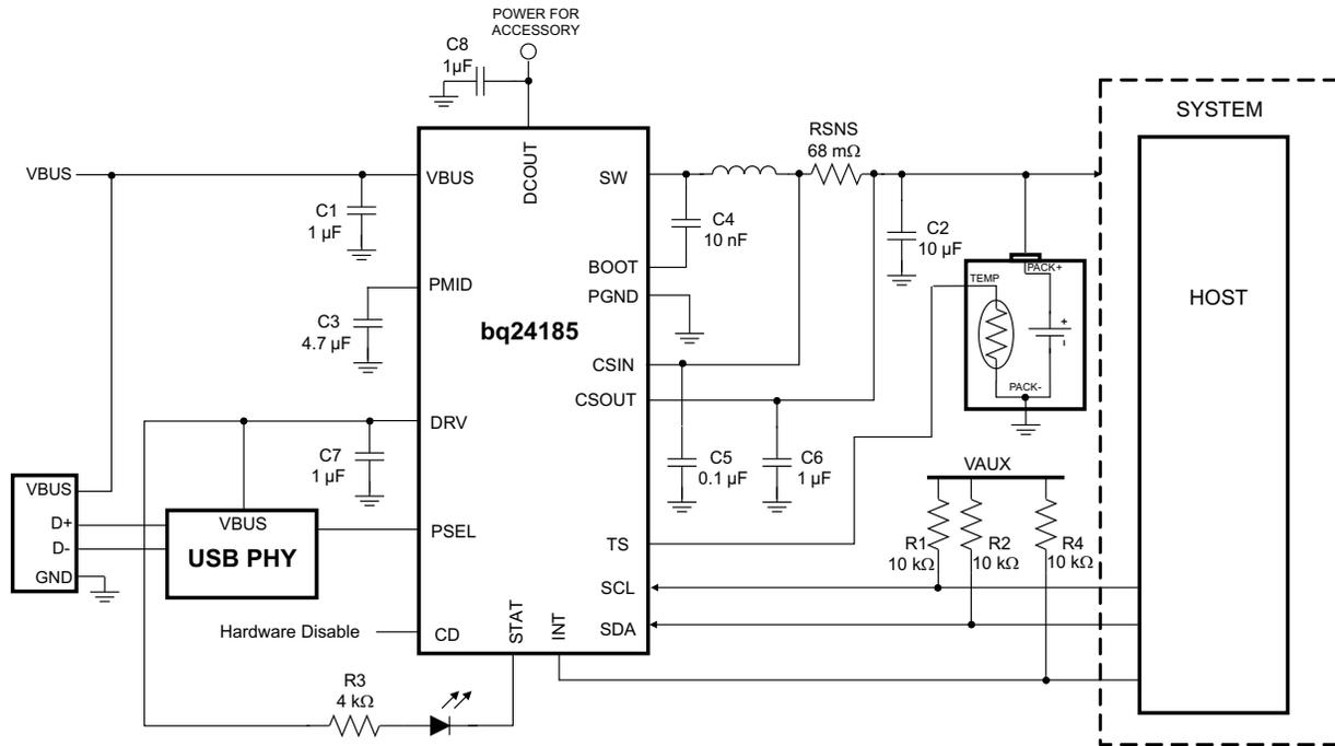
Figure 3. I<sup>2</sup>C Controlled 1-Cell USB Charger Application Circuit
