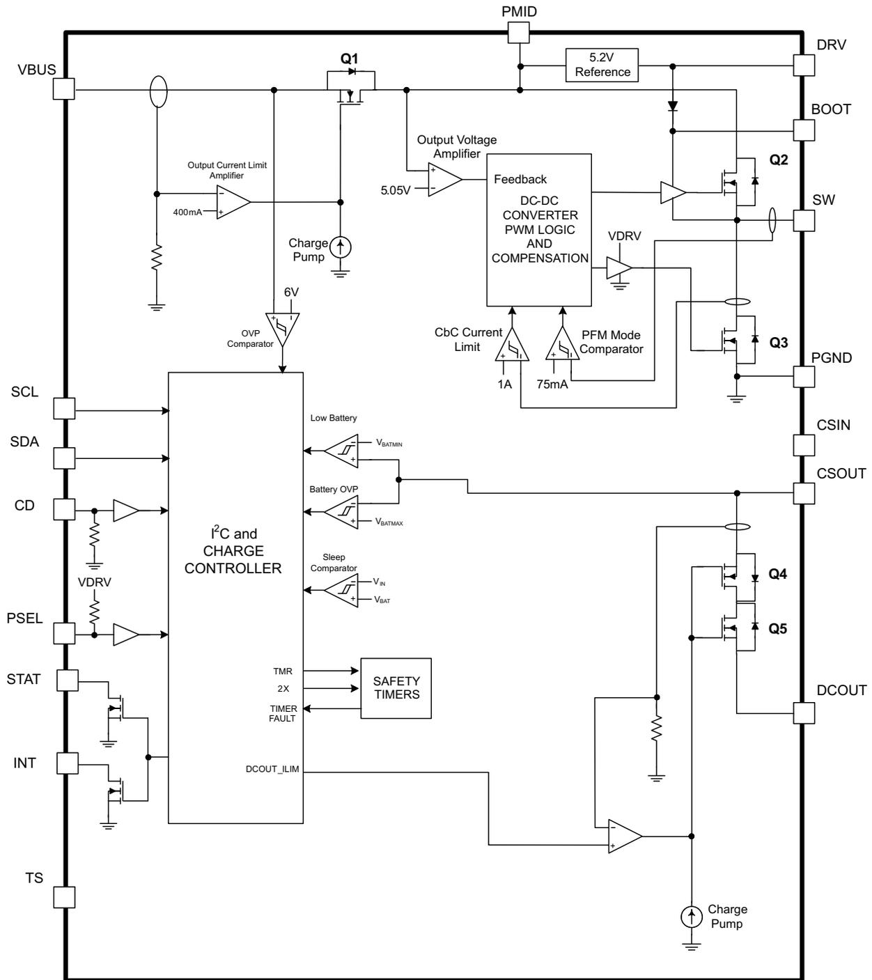
Figure 2. Simplified Block Diagram (Boost Mode, OPA\_MODE = 1)
