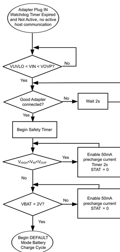
Figure 26. Startup on Adapter Plug-In in DEFAULT Mode
