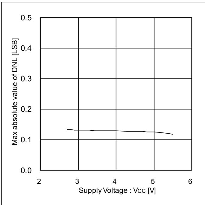
Figure 7. Max absolute value of DNL vs Supply Voltage
