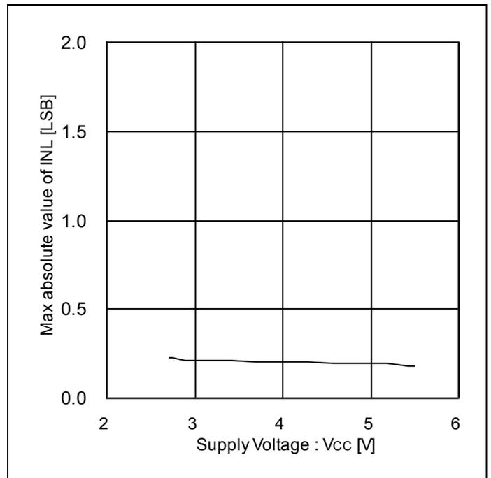
Figure 8. Max absolute value of INL vs Supply Voltage
