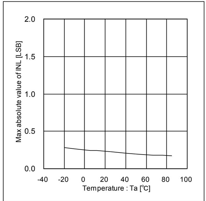
Figure 10. Max absolute value of INL vs Temperature ("Integral Nonlinearity Error", Vcc=3.0V)
