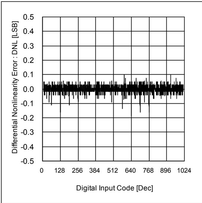
Figure 5. DNL vs Digital Input Code
