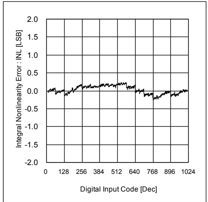
Figure 6. INL vs Digital Input Code
