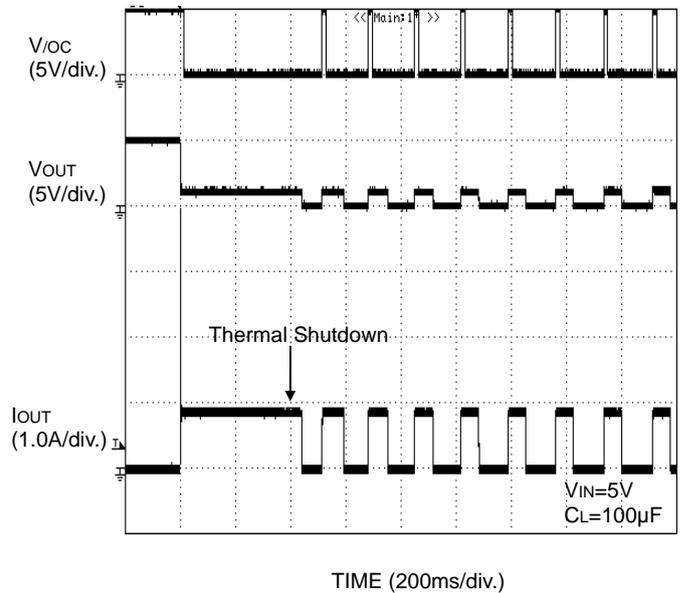
Figure 37. Thermal shutdown 1Ω load connected at enable
