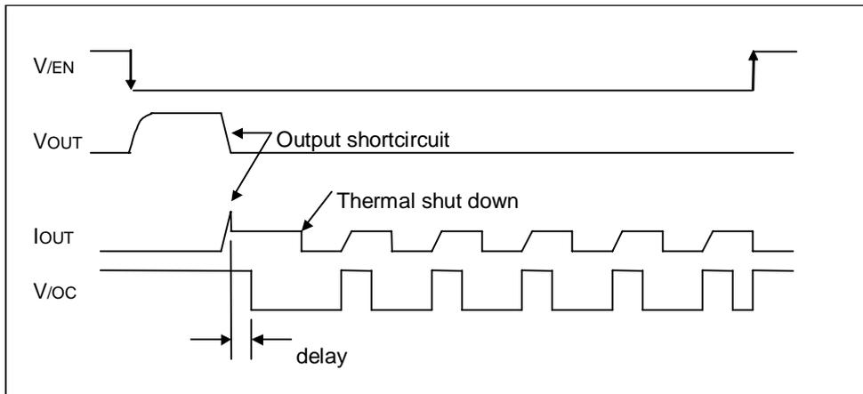
Figure 40. Over-current detection, thermal shutdown timing (BD82000FVJ)
