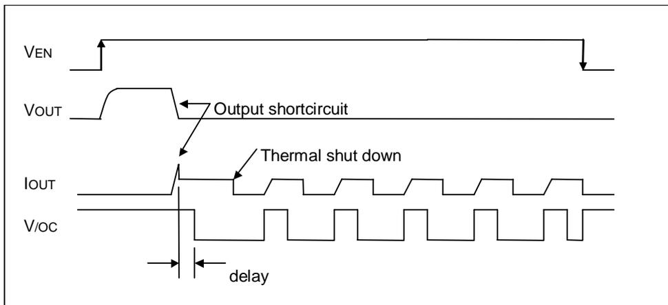
Figure 41. Over-current detection, thermal shutdown timing (BD82001FVJ)
