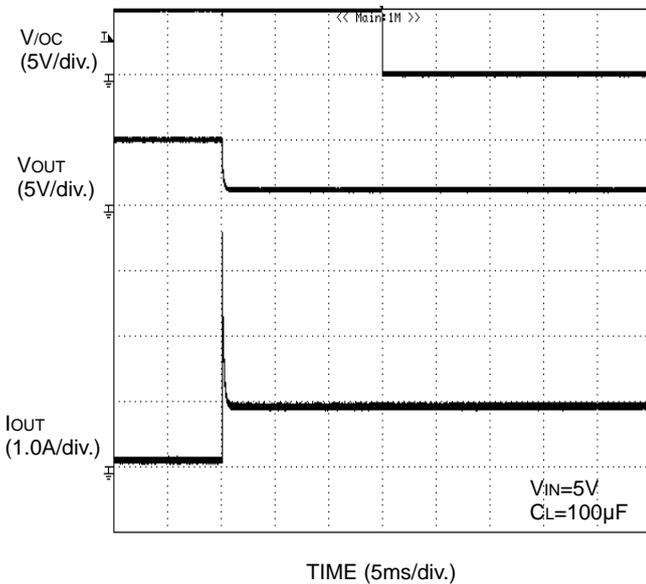
Figure 36. Over-current response 1Ω load connected at enable
