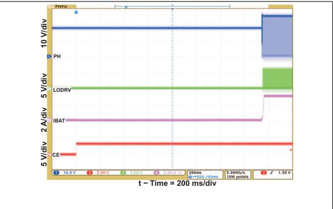
Figure 2. Charge Enable
