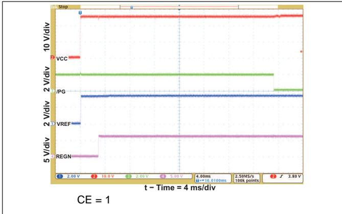
Figure 1. REF REGN and  $\overline{PG}$  Power Up
