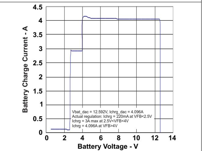
Figure 7. Charge Current Regulation vs VFB Voltage
