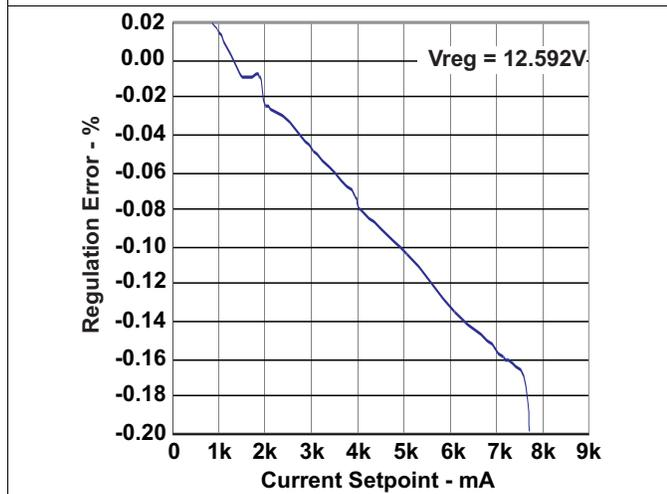
Figure 4. VFB Voltage Regulation Accuracy vs Charge Current
