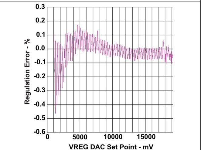
Figure 5. VFB Voltage Regulation Accuracy vs Set Point
