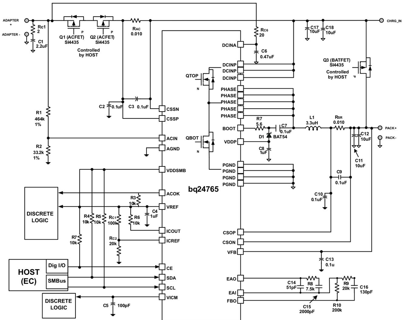
$V_{IN} = 20\text{ V}$ ,  $V_{BAT} = 4\text{-cell Li-Ion}$ ,  $I_{CHARGE} = 4.5\text{ A}$ ,  $I_{dpm} = 5\text{ A}$
