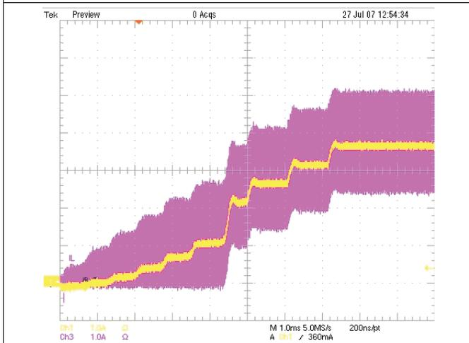
**Figure 22. Inductor Current and Battery Current Soft-Start**
