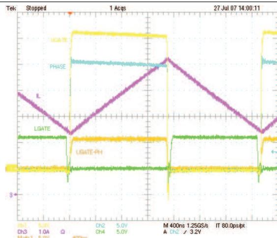
**Figure 23. Continuous Conduction Mode (CCM) Switching Waveforms**
