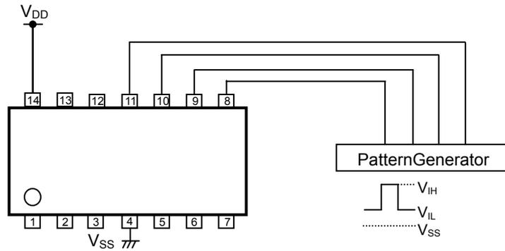
Figure 2. Test Circuit of Input H/L Voltage
