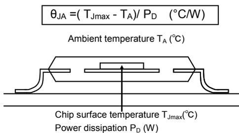
Figure 8. Thermal resistance
