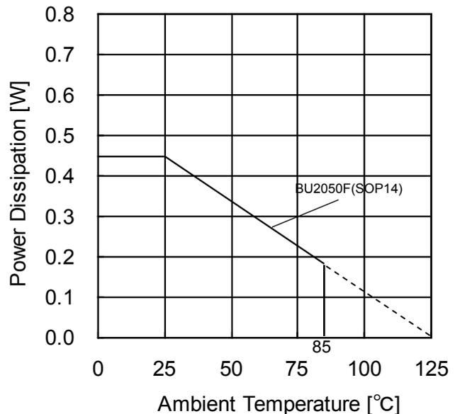
Figure 9. Derating Curve
