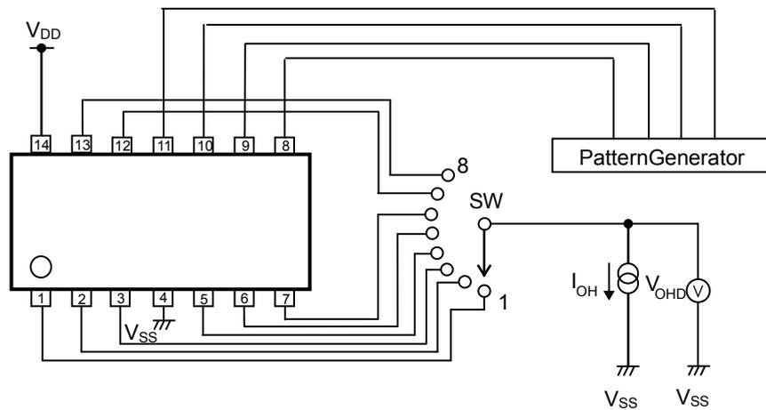
Figure 3. Test Circuit of Output H Voltage
