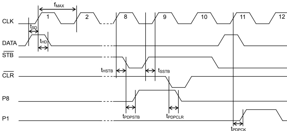
Figure 1. Waveform of Switching Characteristics
