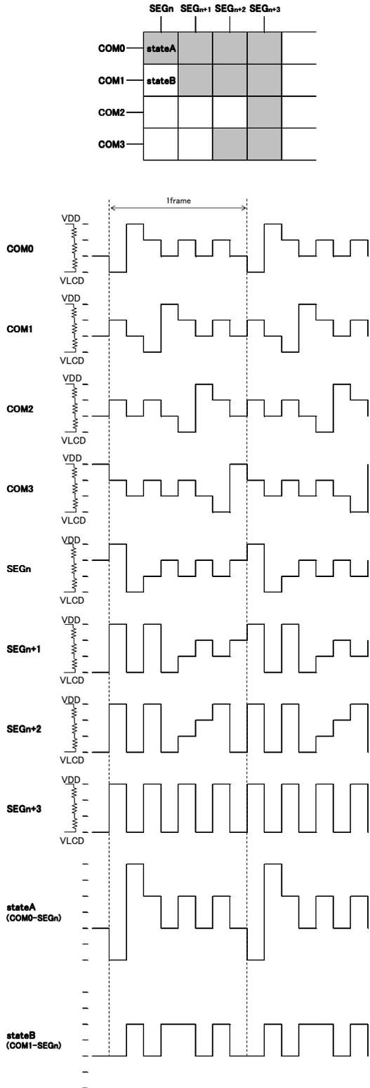
Figure 14. Line inversion waveform(1/3bias)
