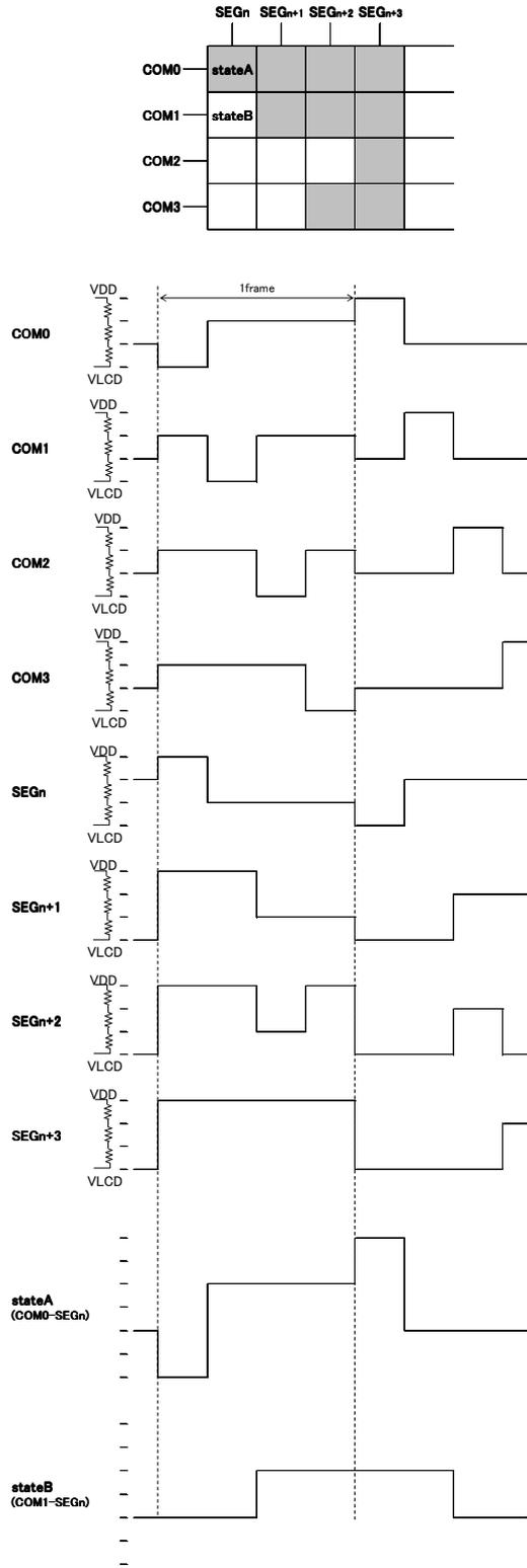
Figure 15. Frame inversion waveform(1/3bias)
