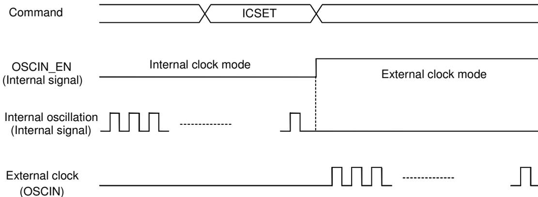
Figure 13. OSCMODE switching timing
