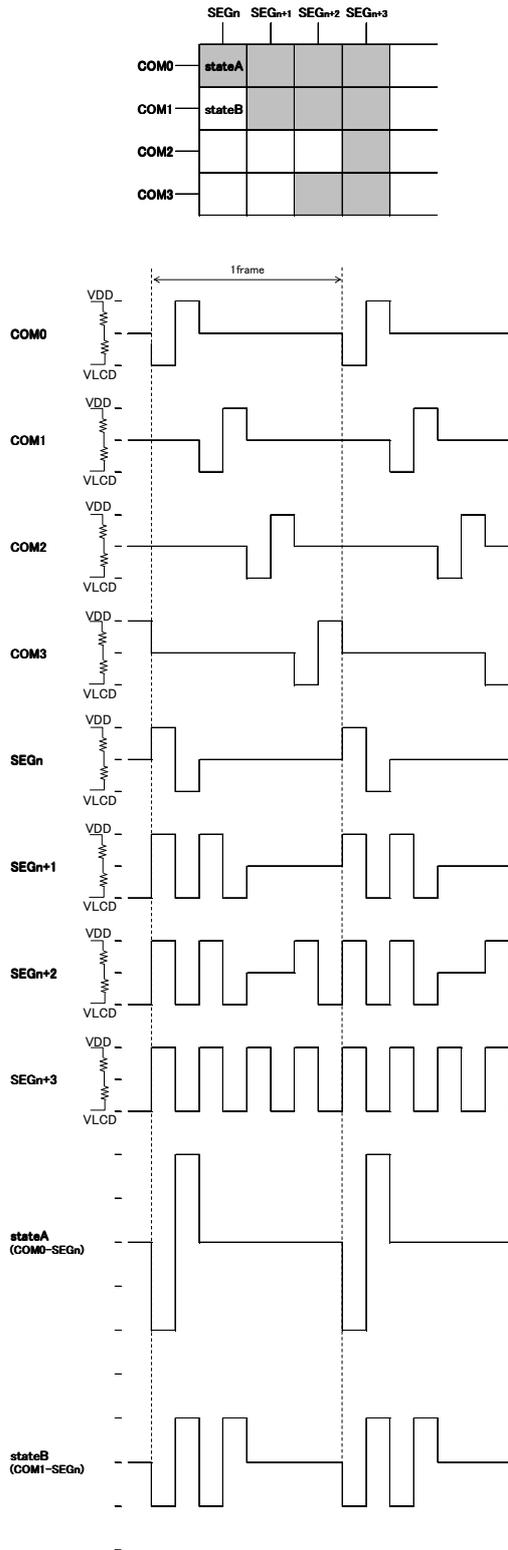
Figure 16. Line inversion waveform(1/2bias)
