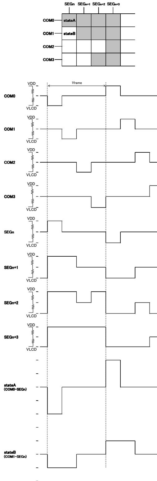
Figure 17. Frame inversion waveform(1/2bias)
