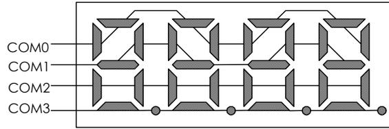
Figure 18. Example COM line pattern
