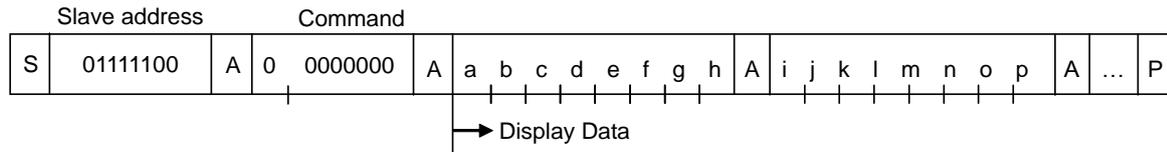
8 bit data will be stored in DDRAM. The address to be written is the address specified by ADSET command, and the address is automatically incremented in every 4bit data.
