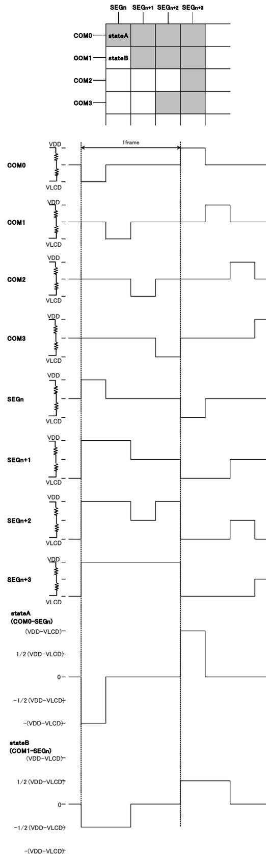
Figure 19. LCD waveform in frame inversion (1/2bias)
