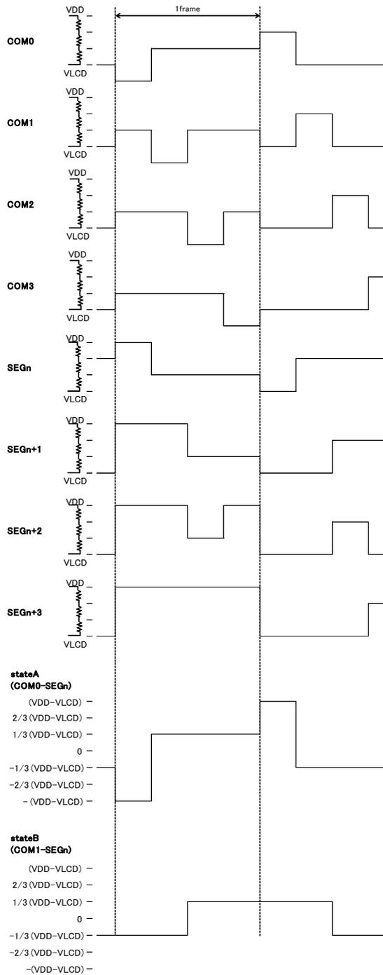
Figure 16. LCD waveform at line inversion (1/3bias)
