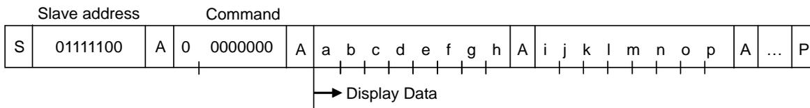
8 bit data will be stored in DDRAM. The address to be written is the address specified by ADSET command, and the address is automatically incremented in every 4bit data.
