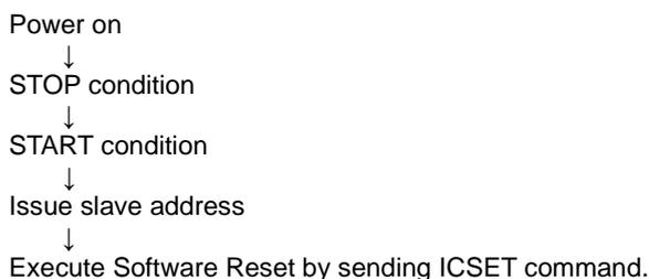
\*Each register value and DDRAM address, DDRAM data are random condition after power on till initialize sequence is executed.
