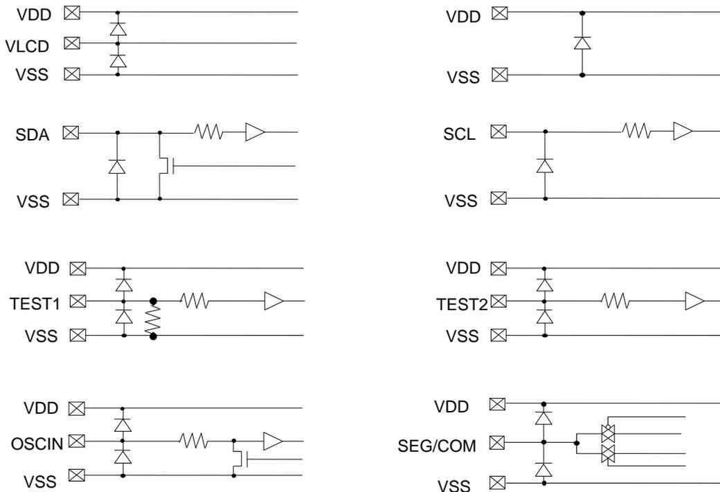
Figure7. I/O equivalent circuit
