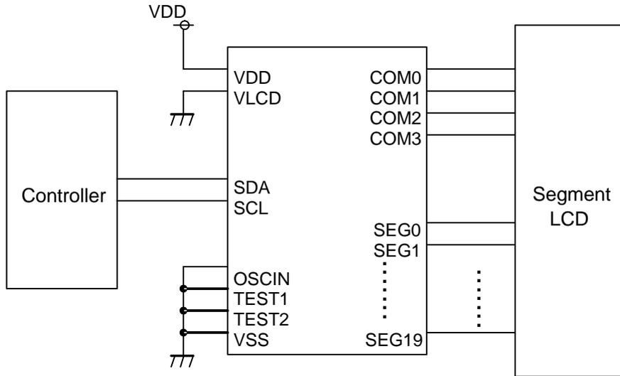
Internal Oscillator circuit use mode
