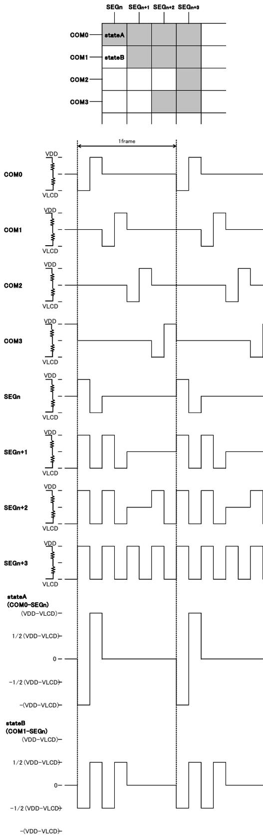
Figure 18. LCD waveform in line inversion (1/2bias)
