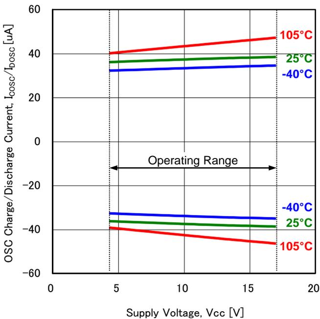
Figure 15. OSC Charge/Discharge Current vs Supply Voltage
