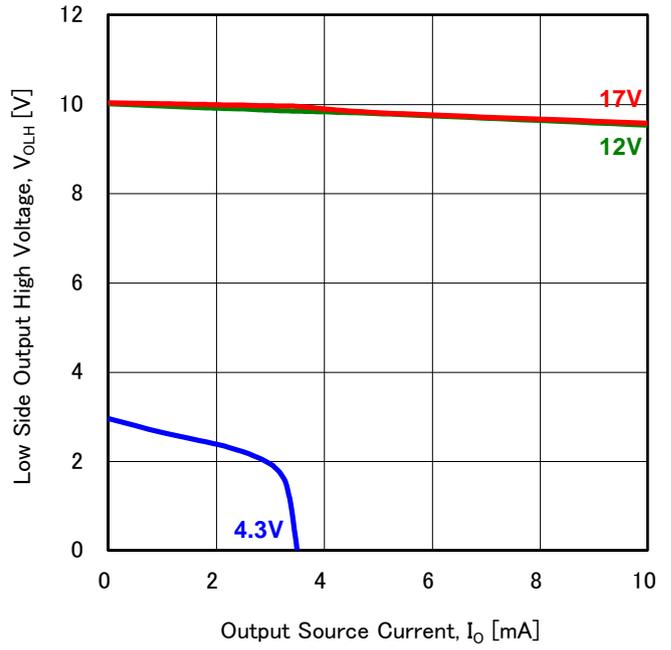
Figure 6. Low Side Output High Voltage vs Output Source Current (T<sub>a</sub>=25°C)
