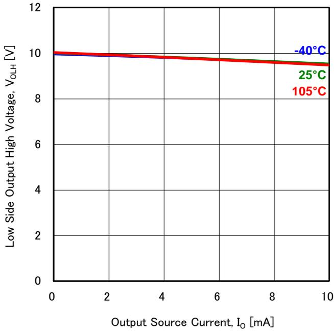
Figure 5. Low Side Output High Voltage vs Output Source Current (V<sub>cc</sub>=12V)
