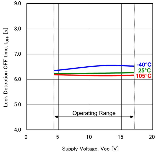
Figure 10. Lock Detection OFF Time vs Supply Voltage
