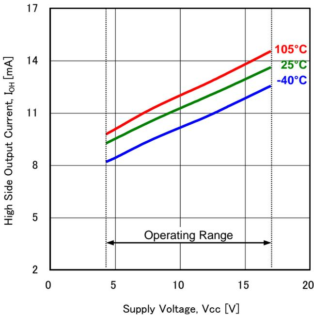
Figure 3. High Side Output Current vs Supply Voltage
