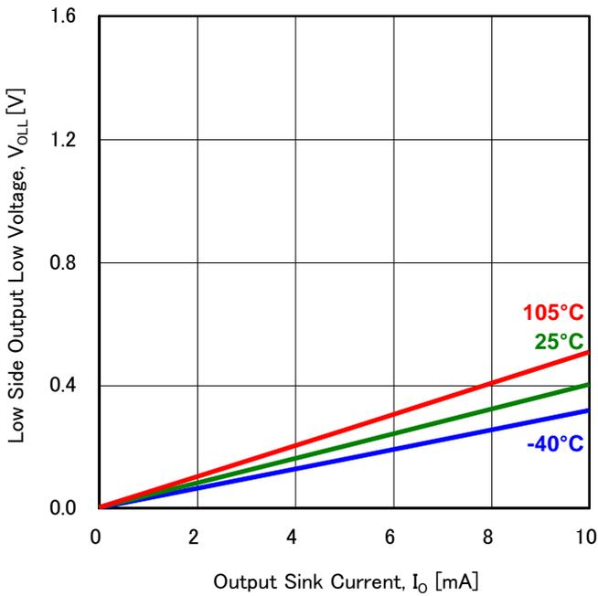
Figure 7. Low Side Output Low Voltage vs Output Sink Current (V<sub>cc</sub>=12V)
