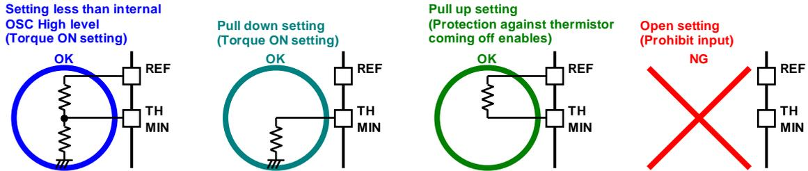
Figure 35. Setting of the variable speed function
