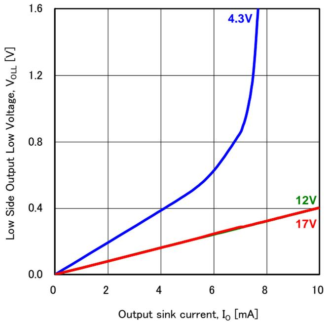
Figure 8. Low Side Output Low Voltage vs Output Sink Current (T<sub>a</sub>=25°C)
