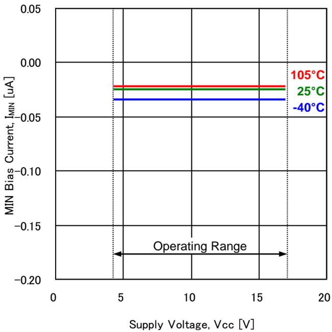
Figure 23. MIN Bias Current vs Supply Voltage
