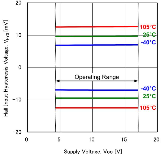
Figure 2. Hall Input Hysteresis Voltage vs Supply Voltage
