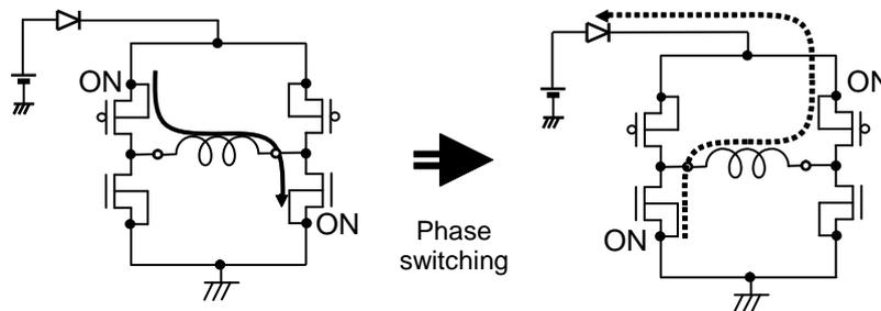
Figure 49. VCC Voltage Rise by Back Electromotive Force
