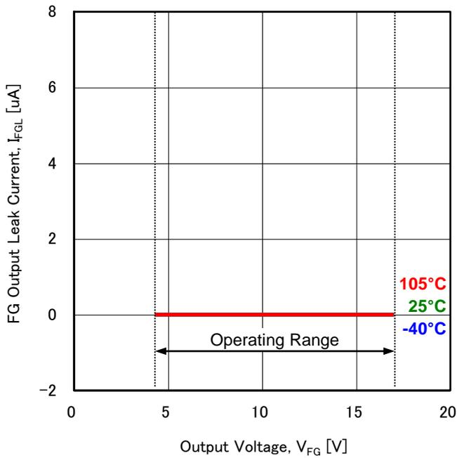
Figure 13. FG Output Leak Current vs Output Voltage
