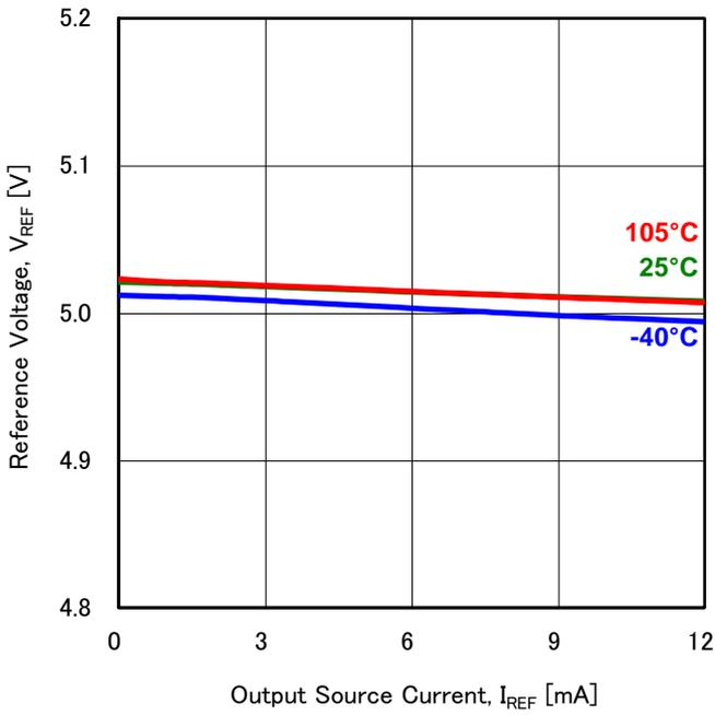
Figure 17. Reference Voltage vs Output Source Current (V<sub>CC</sub>=12V)
