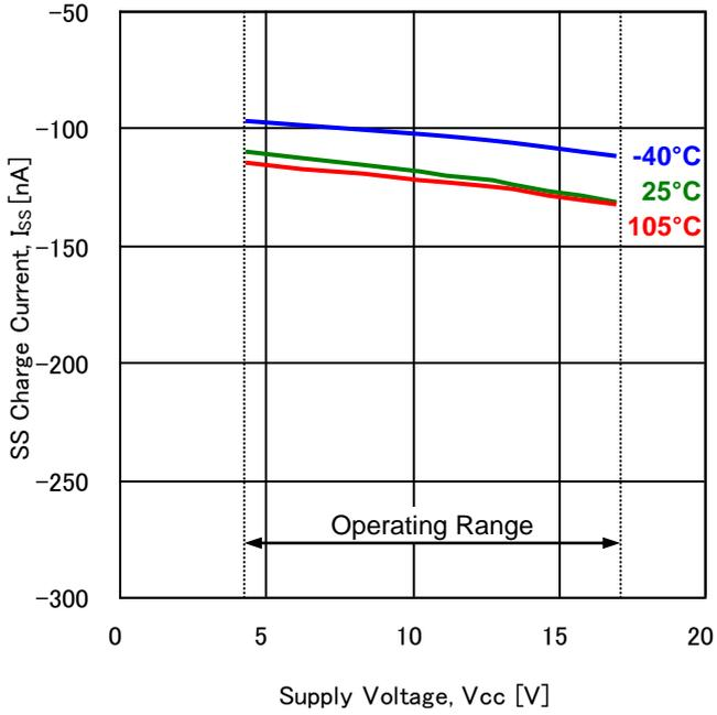
Figure 21. SS Charge Current vs Supply Voltage
