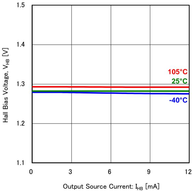
Figure 19. Hall Bias Voltage vs Output Source Current (V<sub>CC</sub>=12V)
