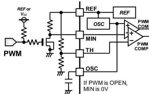
Figure 37. PWM input application 2
