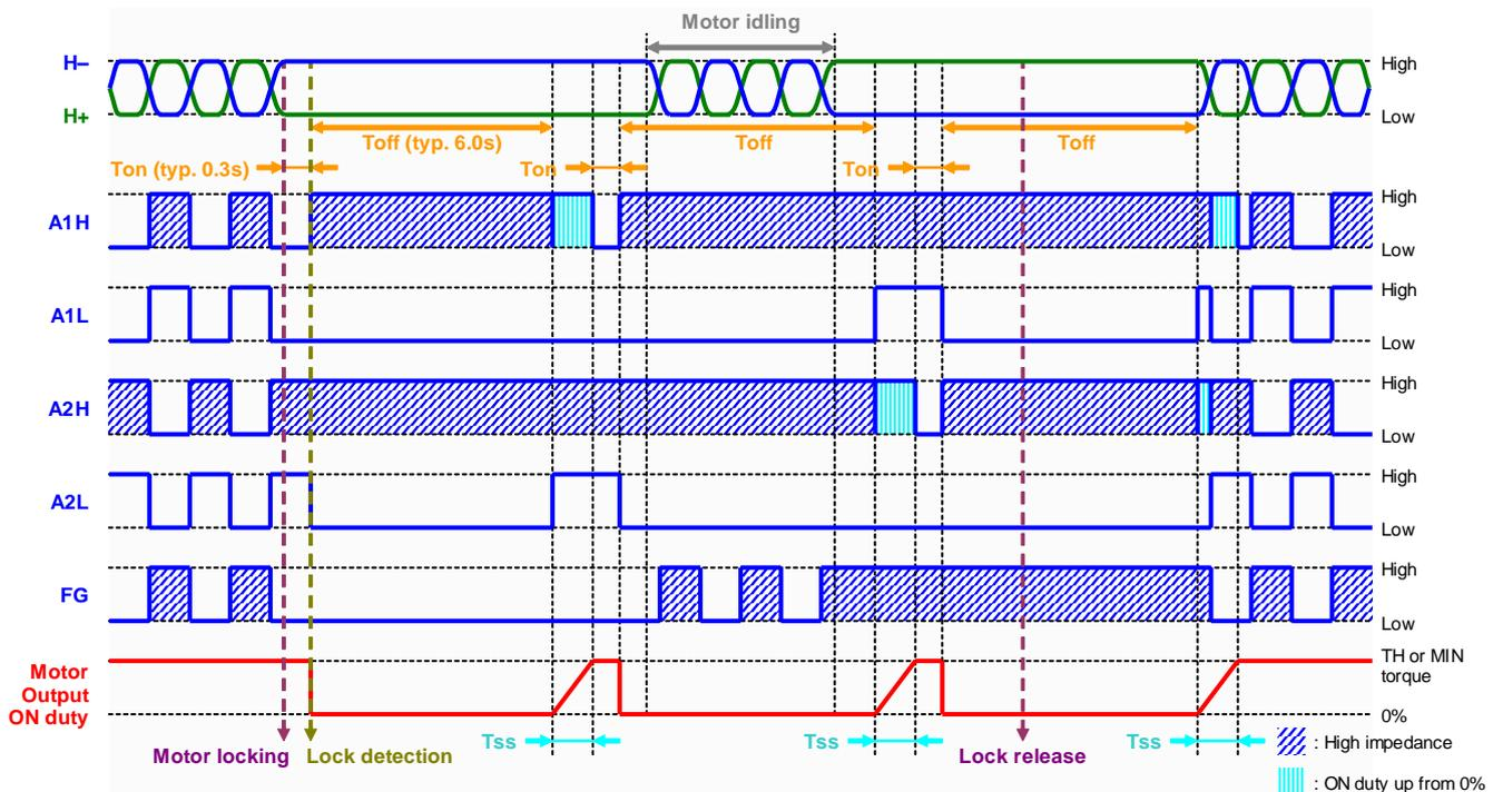
Figure 46. Lock protection (incorporated counter system) timing chart
