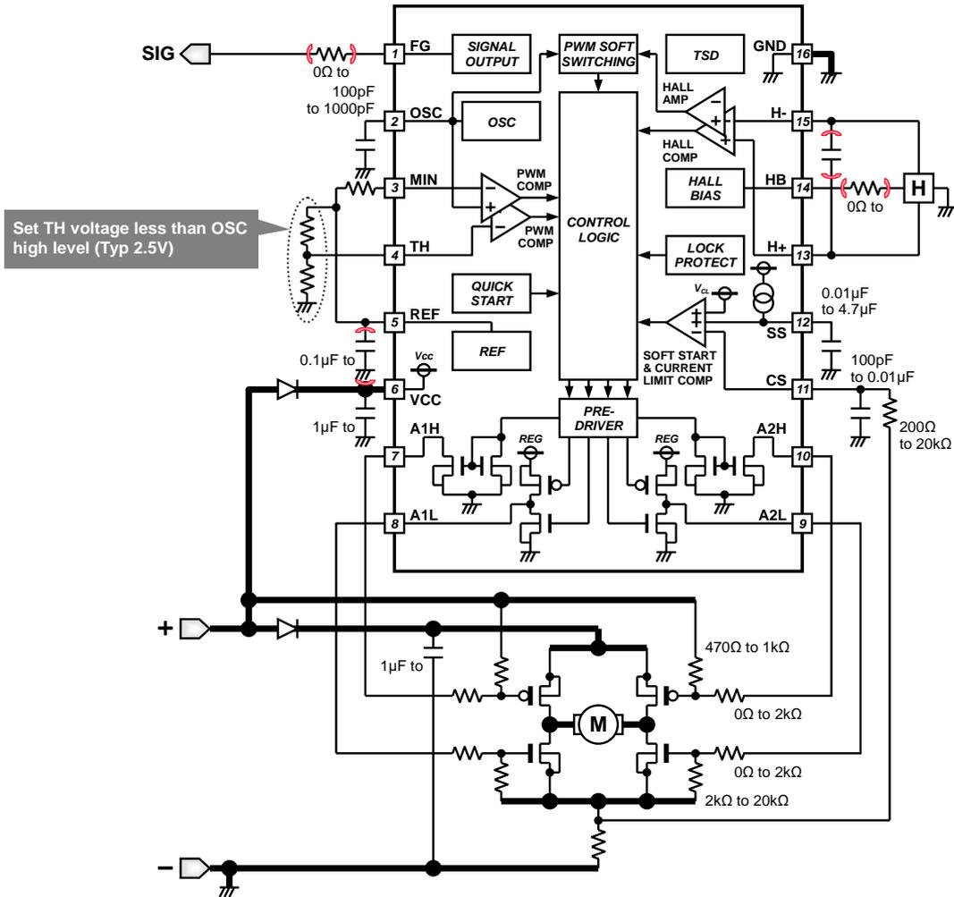
Figure 27. Application of DC voltage input
