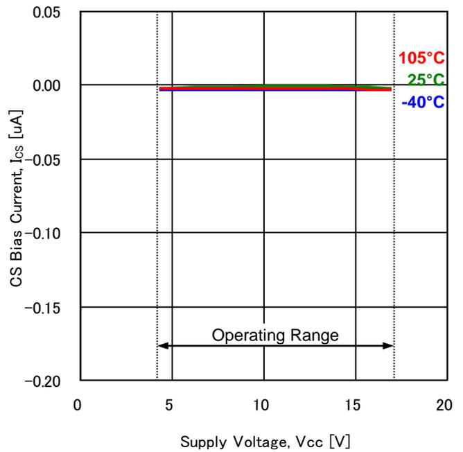
Figure 24. CS Bias Current vs Supply Voltage
