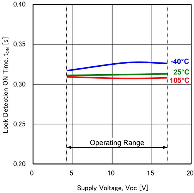
Figure 9. Lock Detection ON Time vs Supply Voltage
