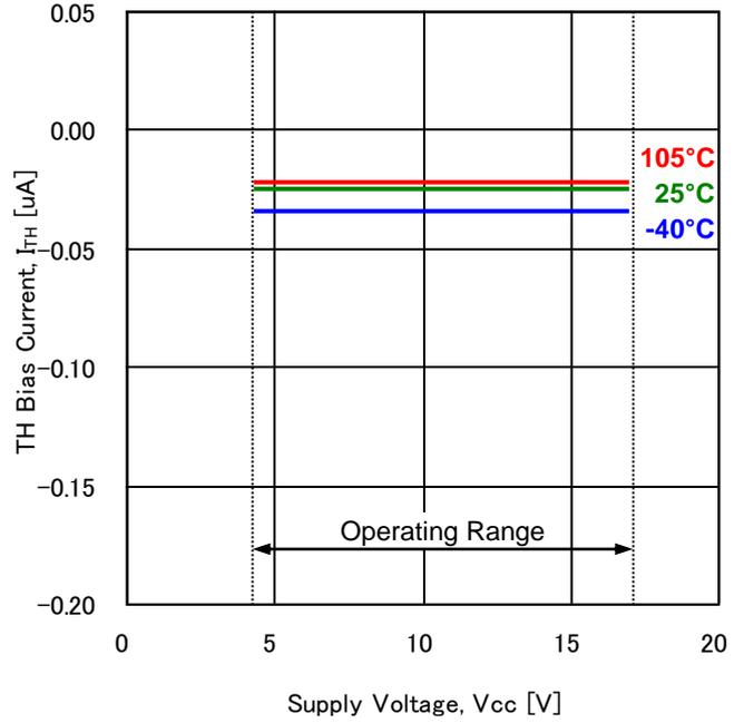
Figure 22. TH Bias Current vs Supply Voltage
