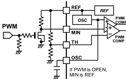
Figure 36. PWM input application 1
