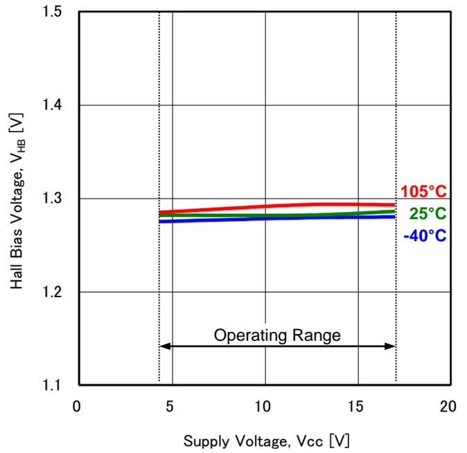
Figure 18. Hall Bias Voltage vs Supply Voltage
