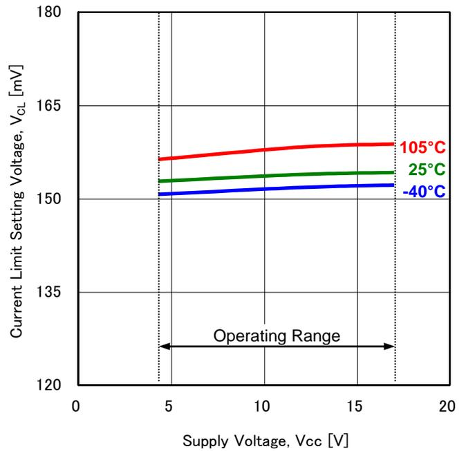
Figure 20. Current Limit Setting Voltage vs Supply Voltage
