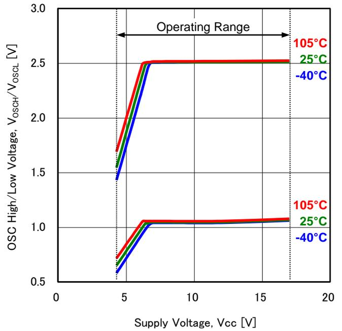
Figure 14. OSC High/Low Voltage vs Supply Voltage
