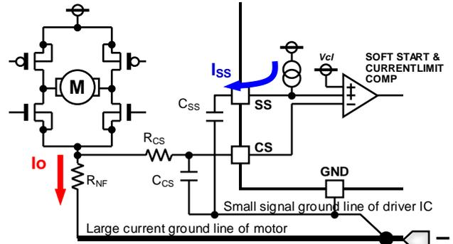
Figure 39. Setting of current limit and ground line
