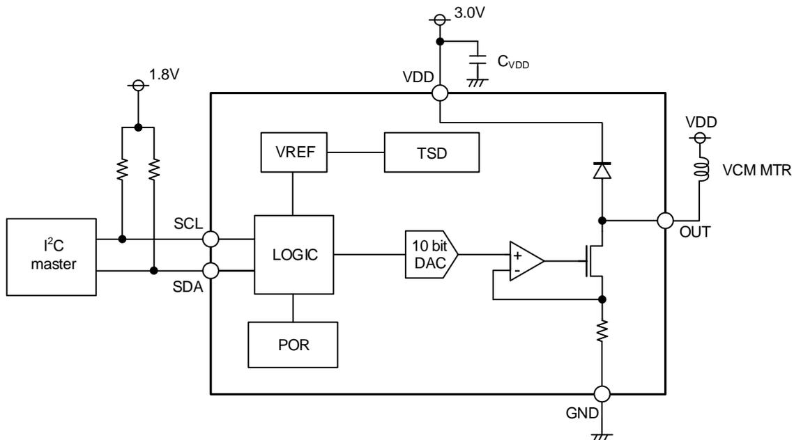
○Product structure : Silicon monolithic integrated circuit ○This product has no designed protection against radioactive rays
