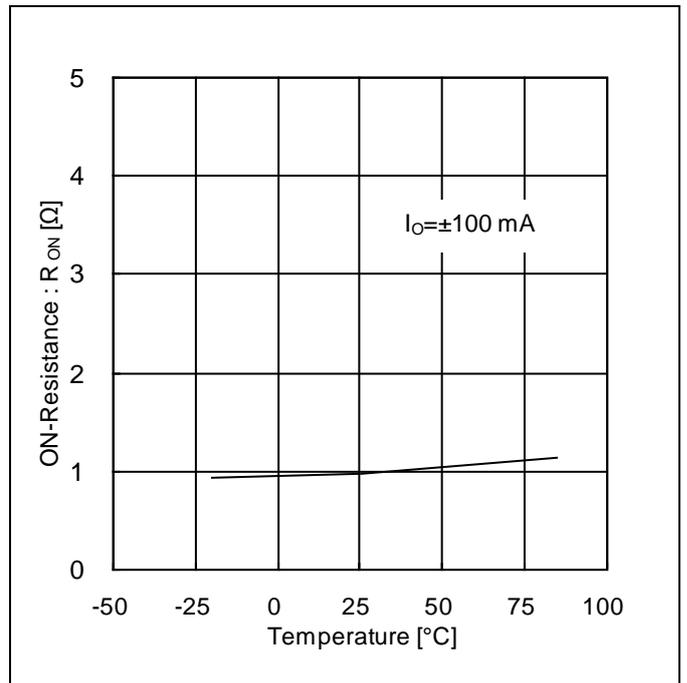
Figure 8. ON-Resistance vs Temperature (Current Driver Block)
