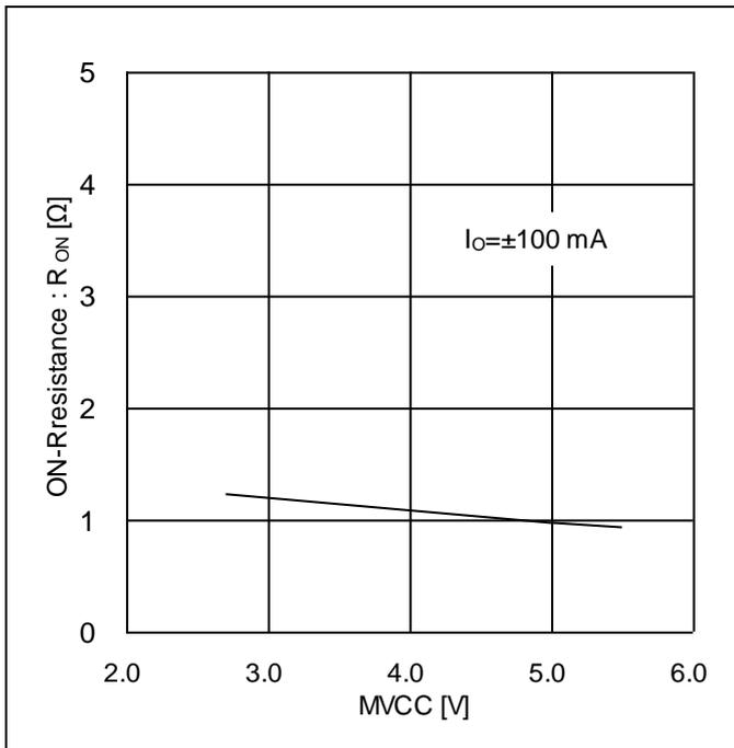
Figure 7. ON-Resistance vs MVCC (Current Driver Block)
