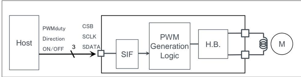
■ Voltage Driver (speed control = ON)
