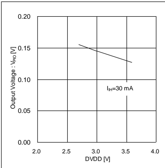
Figure 11. Output Voltage vs DVDD (PI Driver Circuit)
