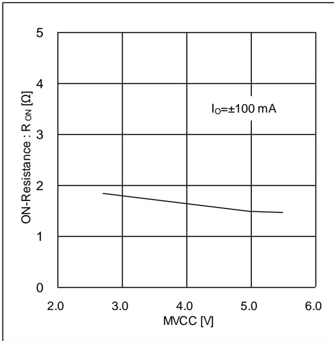
Figure 5. ON-Resistance vs MVCC (Voltage Driver Block)
