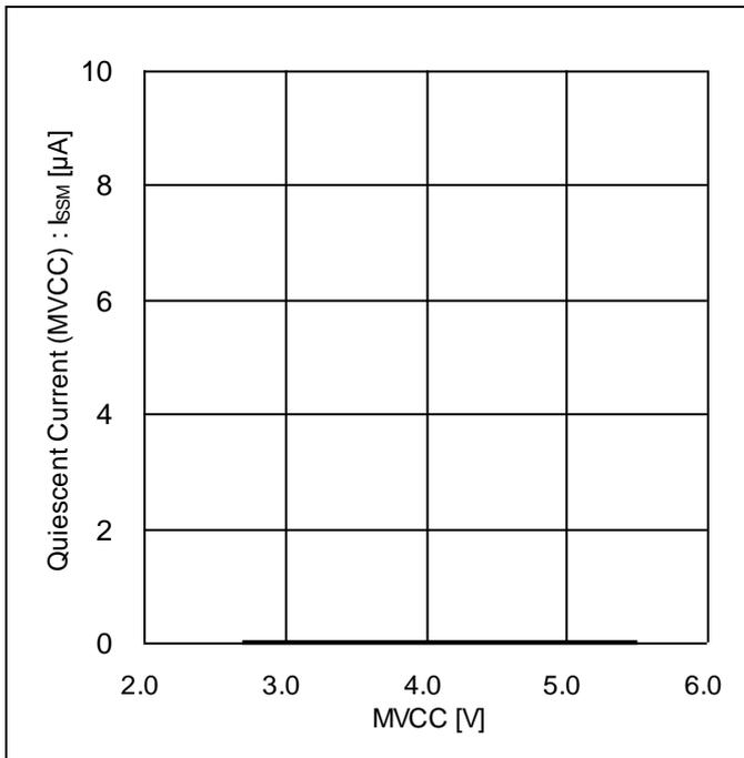
Figure 3. Quiescent Current (MVCC) vs MVCC
