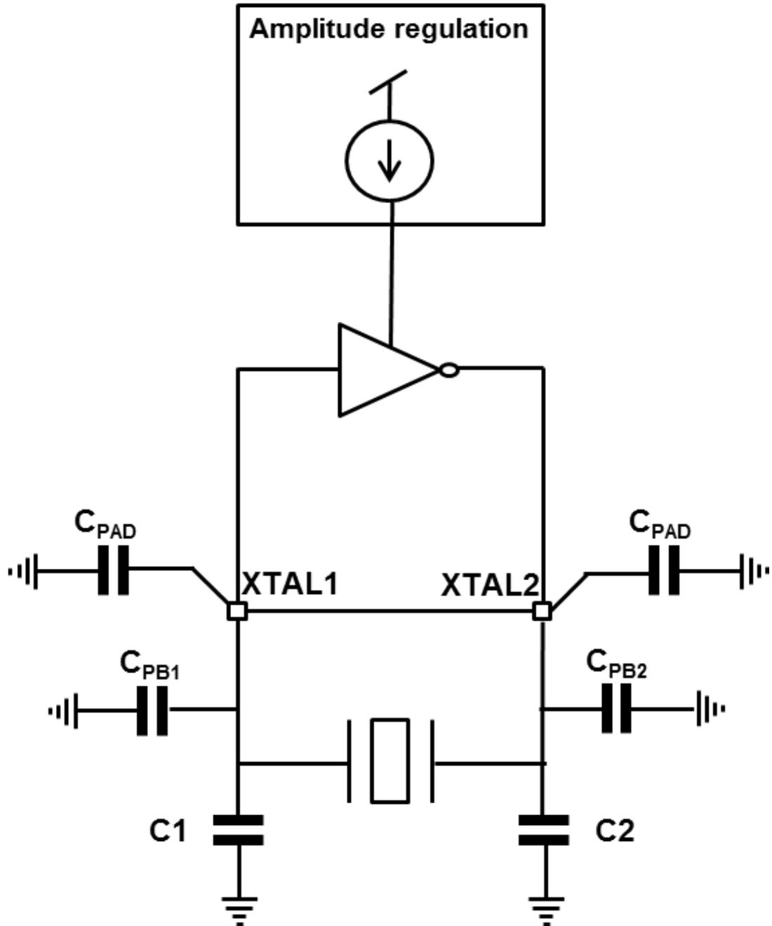
Low power consumption and fast startup time is achieved by choosing a quartz crystal with a low load capacitance C<sub>0</sub>. A reasonable choice for capacitor C<sub>0</sub> is 12 pF. To achieve good frequency stability, the following equation needs to be satisfied:
