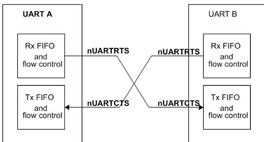
When the RTS flow control is enabled, the UART\_RTS signal is asserted until the receive FIFO is filled up to the programmed watermark level. When the CTS flow control is enabled, the transmitter can only transmit data when the UART\_CTS signal is asserted.
