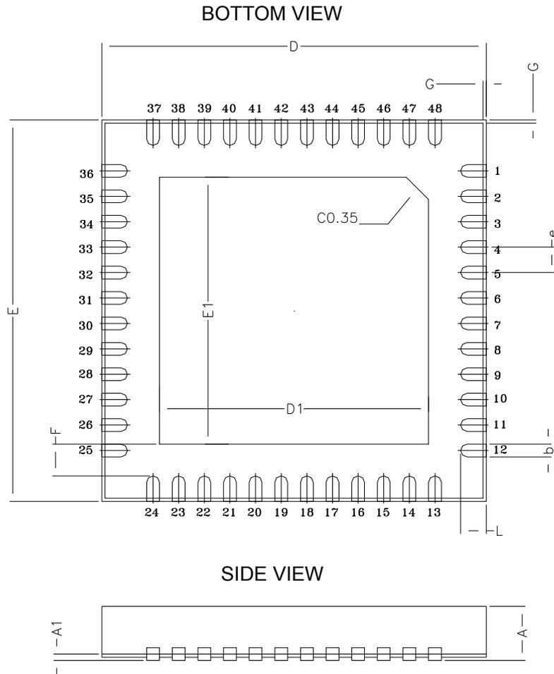
Table 225. QFN48 (|6 x 6 x 0.85 pitch 0.4 mm) mechanical data
