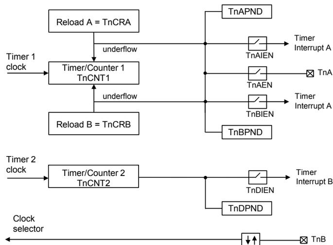
In this mode, the timer toggles the TnA output upon underflow, which is connected to PWMx pin of the device.
