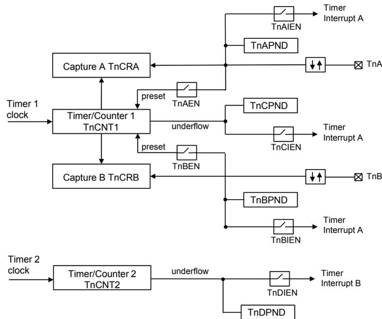
The input signal on TnA and TnB must have a pulse width equal to or greater than one system clock cycle. The value captured in the TnCRA register at different times reflects the elapsed time between transitions on the TnA pin. The same is true for the TnCRB register and TnB pin. Each input pin can be configured to sense either positive edge or negative edge transitions.
