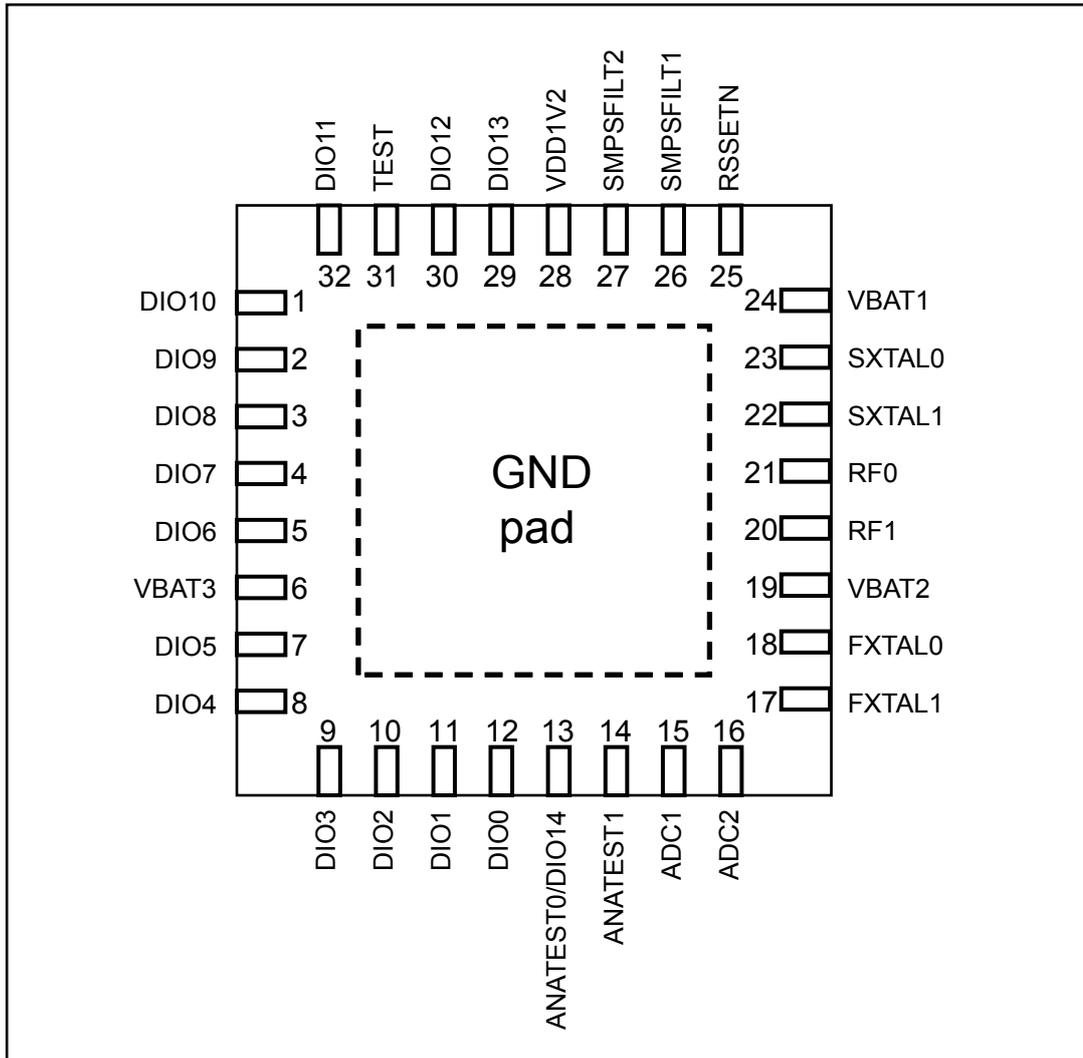
Figure 22. BlueNRG-2 pin out top view (QFN48)
