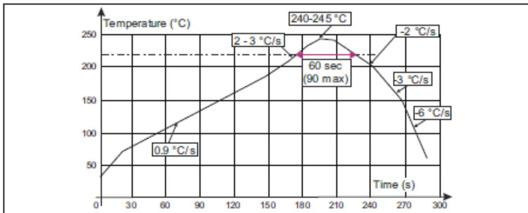
**Table 227. Flip Chip CSP (2.71 x 2.58 x 0.5 pitch 0.4 mm) package reflow profile recommendation**
