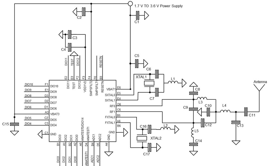
Figure 29. Application circuit: active DC-DC converter QFN32 package with BALF-NRG-02D3 balun
