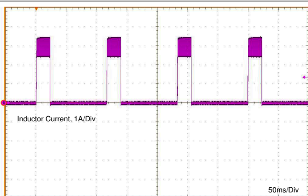
图 8-5. Inductor Current Burst in Short-Circuit Mode
