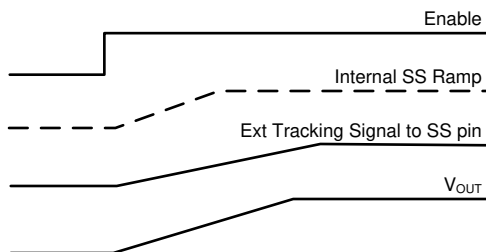
图 10. Tracking with Longer Start-up Time than the Internal Ramp
