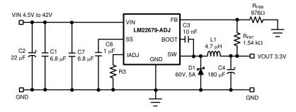
图 8-2. Typical Buck Regulator Application
