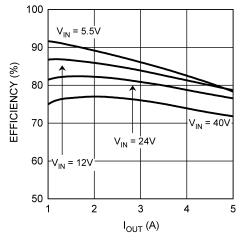
图 8-3. Efficiency vs I<sub>OUT</sub> and V<sub>IN</sub> (V<sub>OUT</sub> = 3.3 V)
