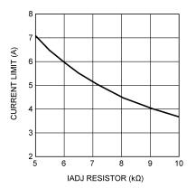
图 7-3. Current Limit vs IADJ Resistor
