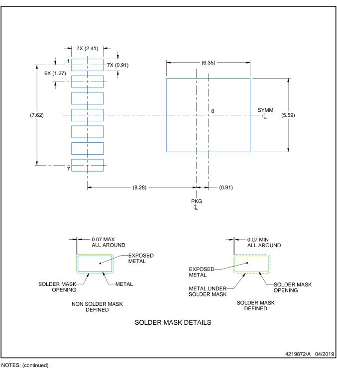
6. This package is designed to be soldered to a thermal pad on the board. For more information, see Texas Instruments literature numbers SLMA002(www.ti.com/lit/slm002) and SLMA004 (www.ti.com/lit/slma004).
