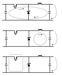
图 10-1. Current Flow in a Buck Application
