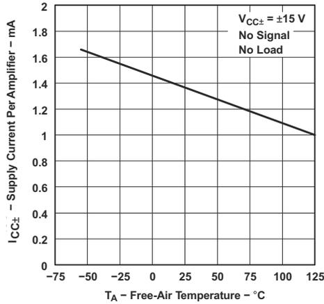
Figure 6-52. Supply Current Per Amplifier vs Free-Air Temperature
