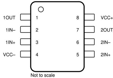
**Figure 5-4. TL072x D, DDF, JG, P, PS, and PW Package
