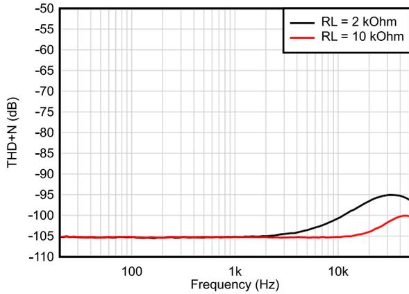
BW = 80 kHz,  $V_{OUT} = 1\text{ V}_{RMS}$
