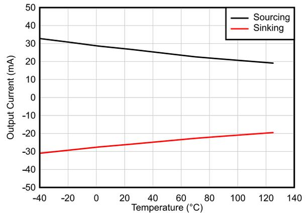
**Figure 6-36. Short-Circuit Current vs Temperature**
