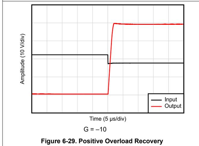
Figure 6-29. Positive Overload Recovery
