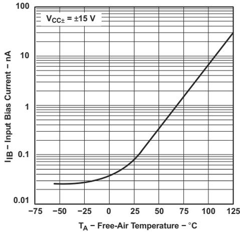
Figure 6-40. Input Bias Current vs Free-Air Temperature
