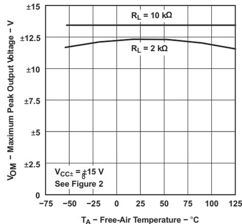
Figure 6-44. Maximum Peak Output Voltage vs Free-Air Temperature
