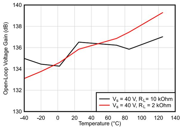
Figure 6-23. Open-Loop Voltage Gain vs Temperature (dB)
