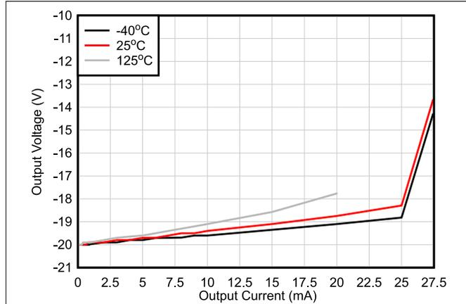
Figure 6-13. Output Voltage Swing vs Output Current (Sinking)
