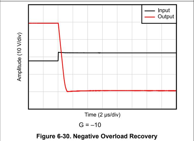
Figure 6-30. Negative Overload Recovery
