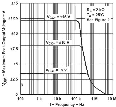
Figure 6-42. Maximum Peak Output Voltage vs Frequency
