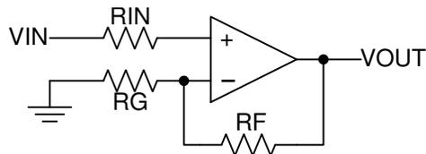
**Figure 11-2. Operational Amplifier Schematic for Noninverting Configuration**
