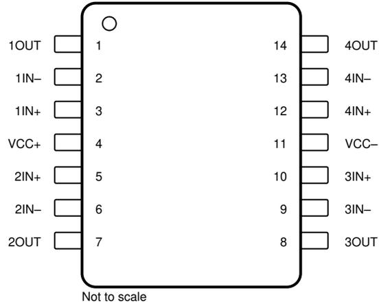
**Figure 5-7. TL074x D, N, NS, PW, J, DYY, and W Package
