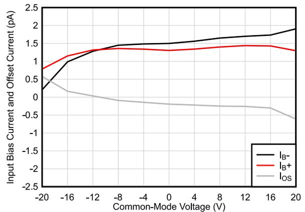
**Figure 6-10. Input Bias Current vs Common-Mode Voltage**
