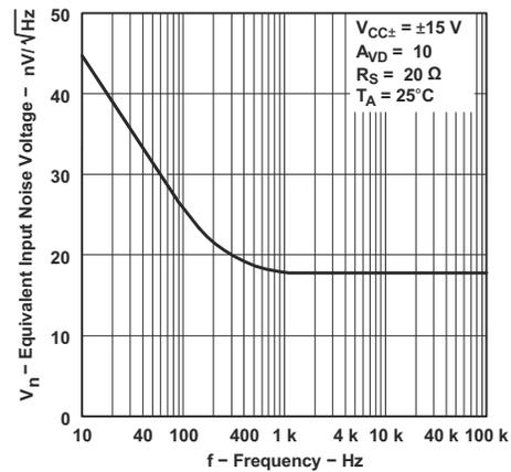
Figure 6-55. Equivalent Input Noise Voltage vs Frequency
