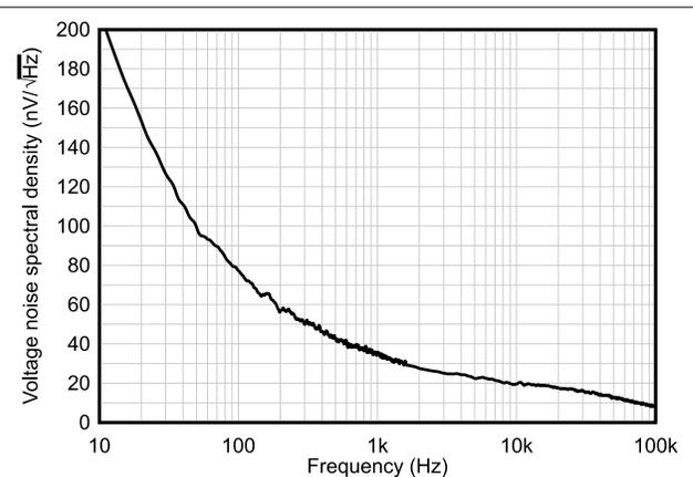
Figure 6-18. Input Voltage Noise Spectral Density vs Frequency
