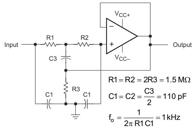
**Figure 9-7. High-Q Notch Filter**
