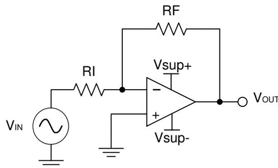
Figure 9-1. Inverting Amplifier
