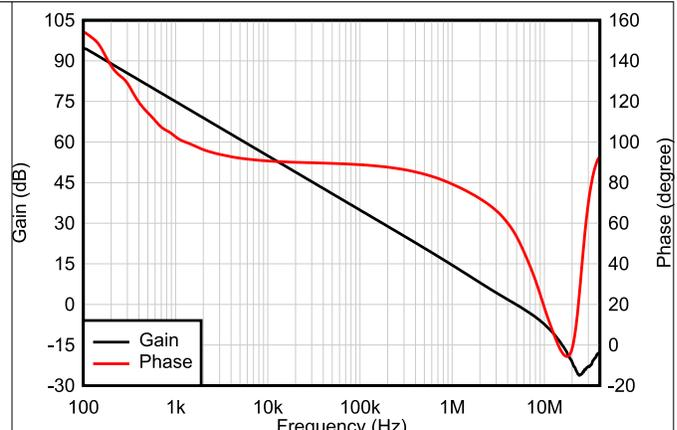
**Figure 6-8. Open-Loop Gain and Phase vs Frequency**
