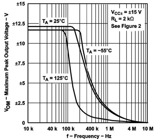
Figure 6-43. Maximum Peak Output Voltage vs Frequency
