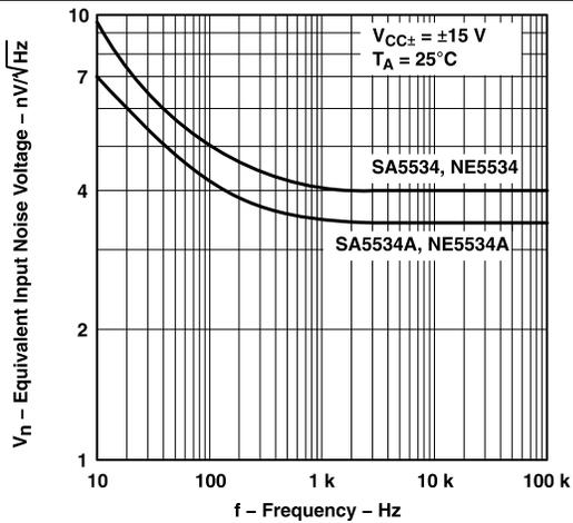
Figure 7. Equivalent Input Noise Voltage vs Frequency
