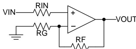
Figure 15. Operational Amplifier Schematic for Noninverting Configuration
