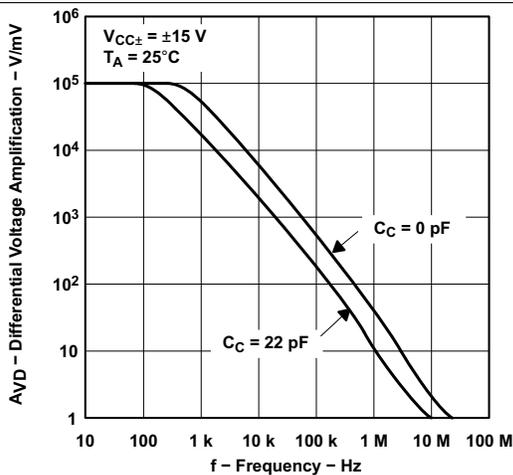
Figure 3. Large-Signal Differential Voltage Amplification vs Frequency
