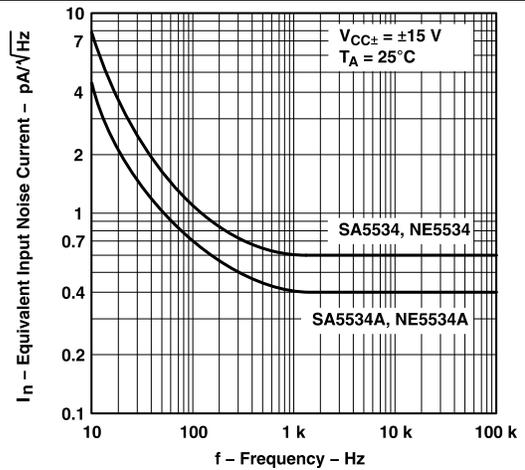
Figure 8. Equivalent Input Noise Current vs Frequency
