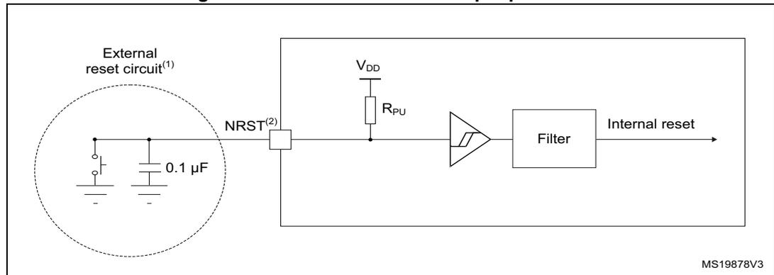
1. The external capacitor protects the device against parasitic resets.
