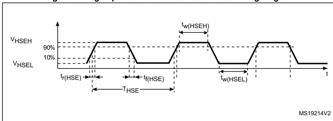
**Low-speed external user clock generated from an external source**
