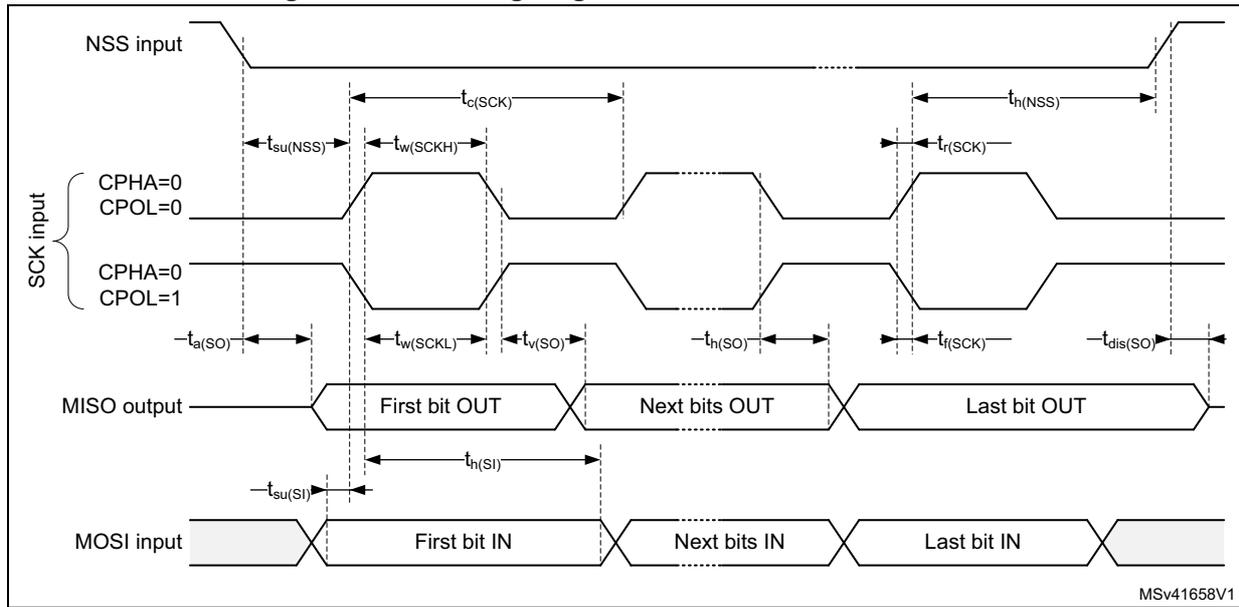
Figure 25. SPI timing diagram - slave mode and CPHA = 1
