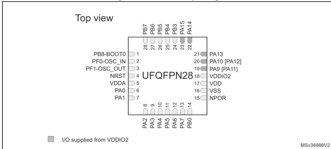
1. Pin pair PA11/12 can be remapped in place of pin pair PA9/10 using the SYSCFG\_CFGR1 register.
