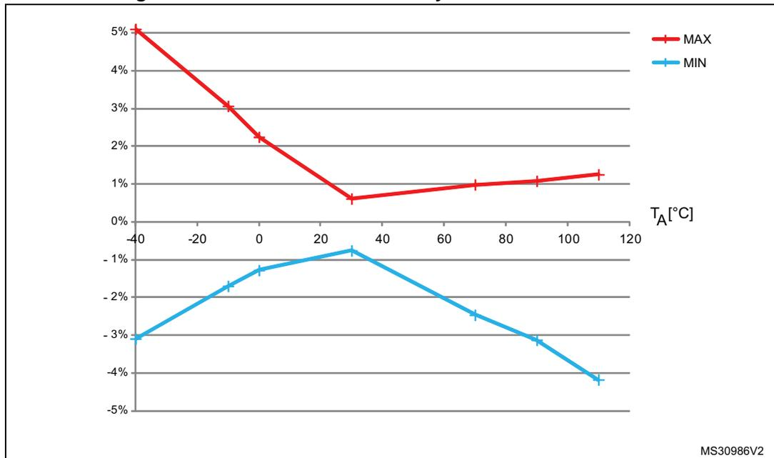
High-speed internal 48 MHz (HSI48) RC oscillator
