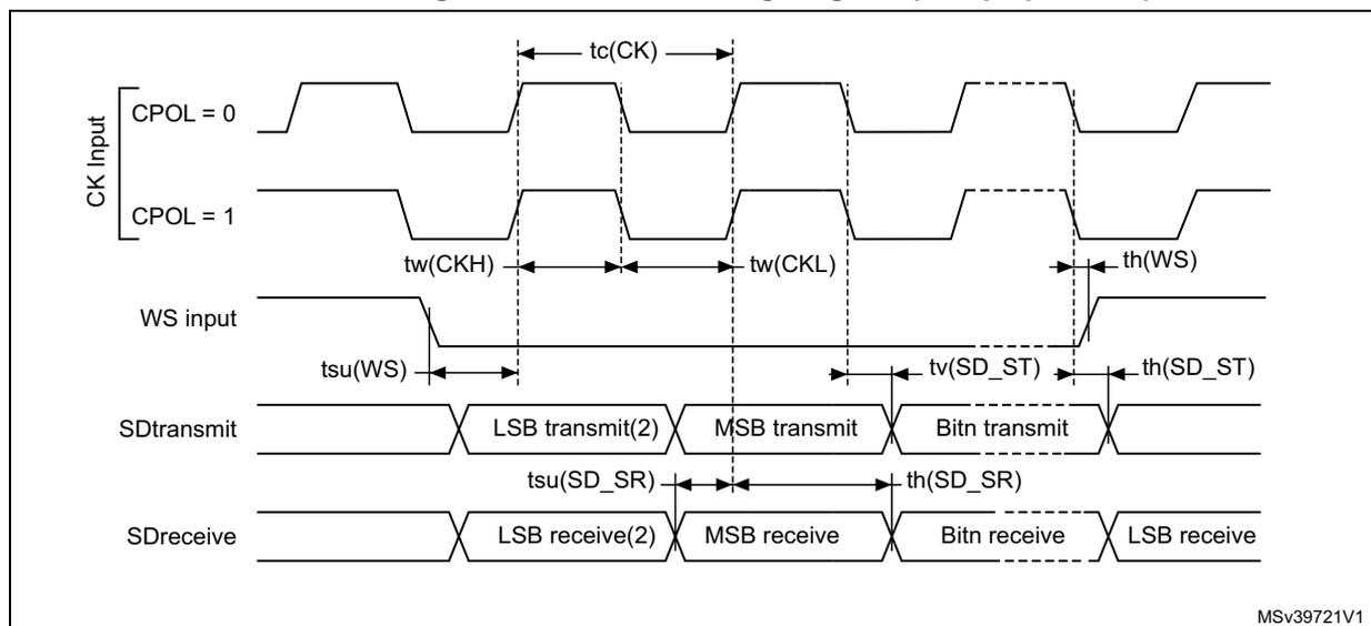
1. Measurement points are done at CMOS levels:  $0.3 \times V_{DDIOx}$  and  $0.7 \times V_{DDIOx}$ .
