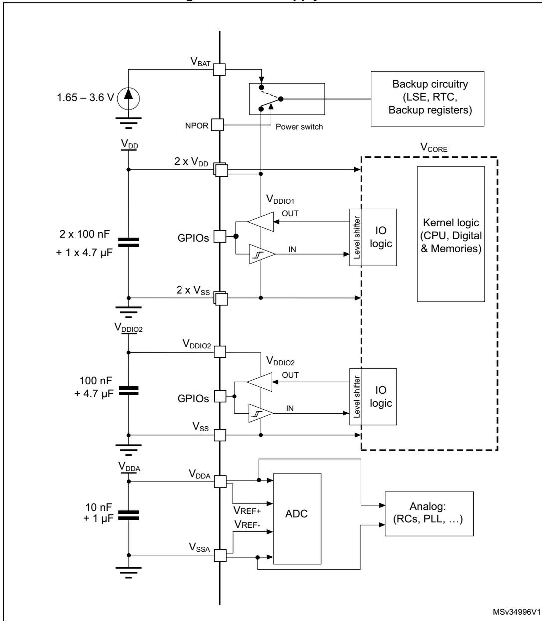
**Caution:** Each power supply pair (V<sub>DD</sub>/V<sub>SS</sub>, V<sub>DDA</sub>/V<sub>SSA</sub> etc.) must be decoupled with filtering ceramic capacitors as shown above. These capacitors must be placed as close as possible to, or below, the appropriate pins on the underside of the PCB to ensure the good functionality of the device.
