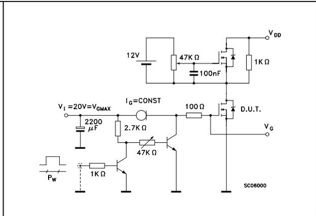
Figure 14. Test circuit for inductive load switching and diode recovery times
