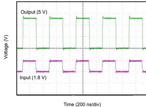
**Figure 5. Translation Up (1.8 V to 5 V) at 2.5 MHz**
