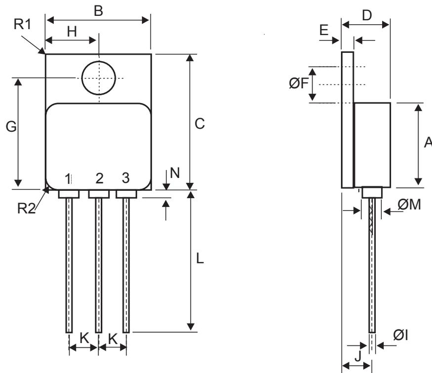
The TO-254-AA is a metallic package. It is not connected to any pin nor to the inside die.
