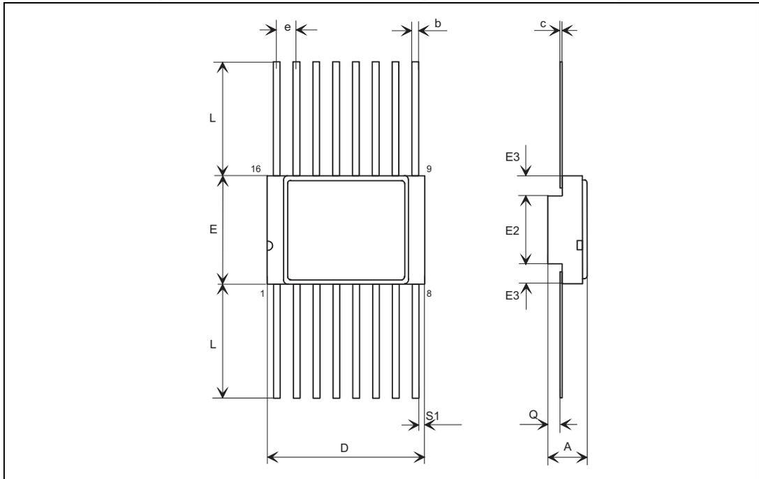
1. The upper metallic lid is electrically connected to ground.
