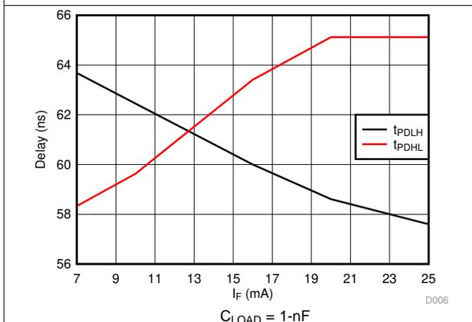
图 8. Propagation delay versus Forward current
