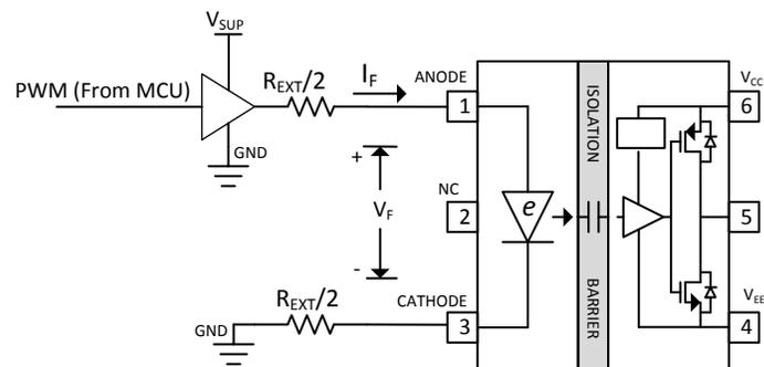
$$R_{EXT} = \frac{V_{SUP} - V_F}{I_F} - R_{OH\_buf}$$
