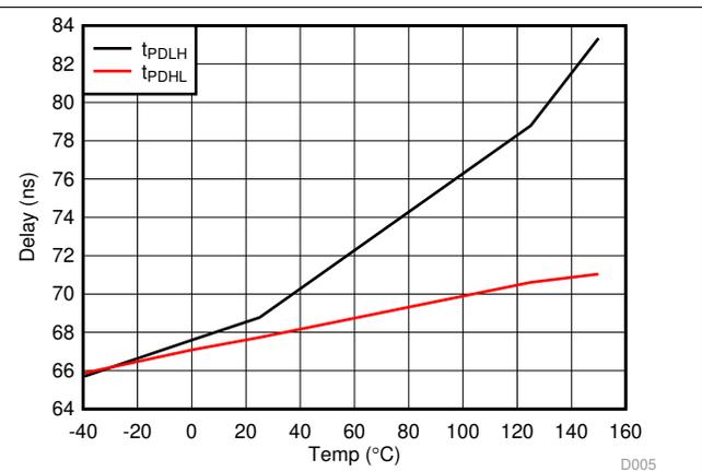
图 7. Propagation delay versus Temperature
