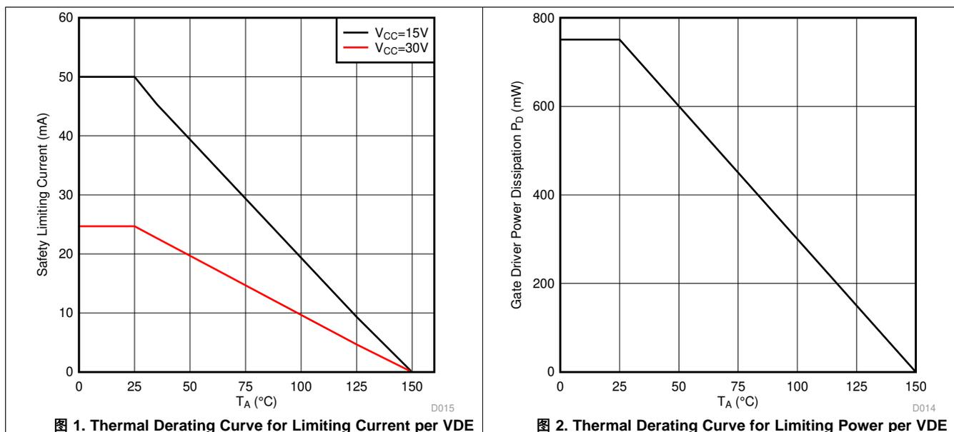
图 1. Thermal Derating Curve for Limiting Current per VDE
