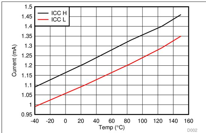
图 4. Supply currents versus Temperature
