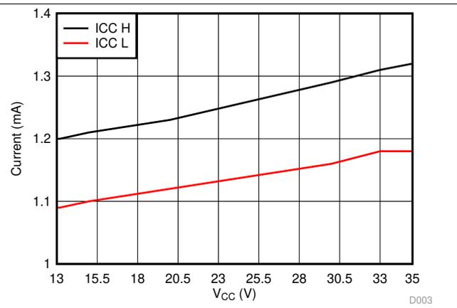
图 5. Supply current versus Supply Voltage
