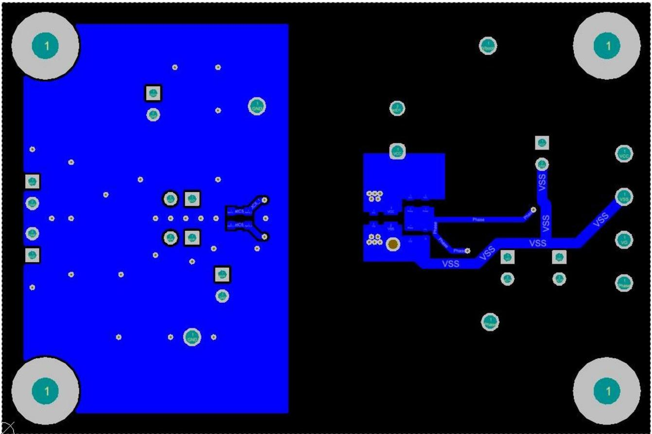
图 33. Bottom-Layer Traces and Copper (Flipped)
