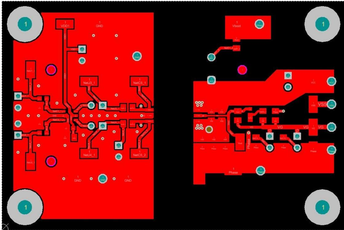
图 32. Top-Layer Traces and Copper
