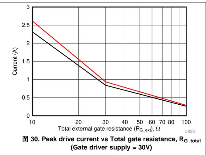
Use 表 6 to find the minimum gate resistance to be used with UCC23511 when driving a power switch. The values shown includes the power switch internal gate resistance  $R_{G\_int}$ . Hence,  $R_{G\_int}$  must be subtracted from the values shown to determine the value of the resistor to populate on the printed circuit board.
