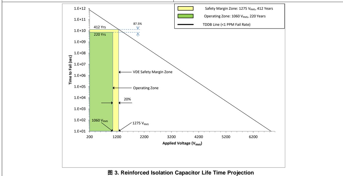
图 3. Reinforced Isolation Capacitor Life Time Projection
