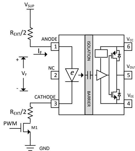
$$R_{EXT} = \frac{V_{SUP} - V_F}{I_F} - R_{M1}$$
