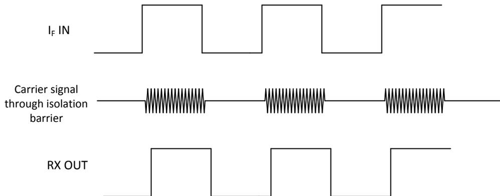
**图 20. On-Off Keying (OOK) Based Modulation Scheme**
