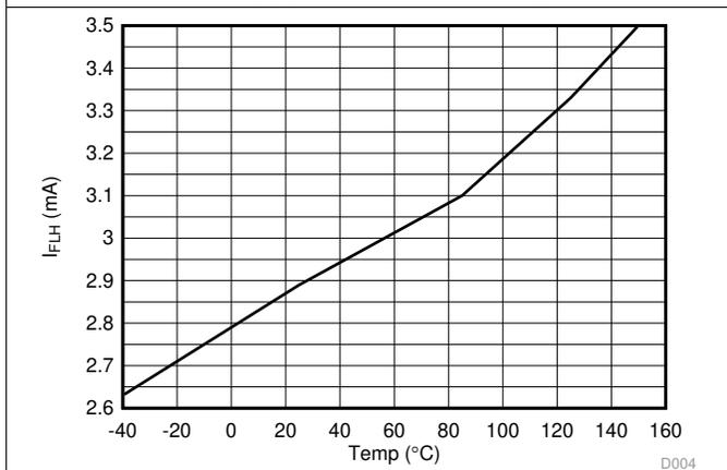
图 6. Forward threshold current versus Temperature
