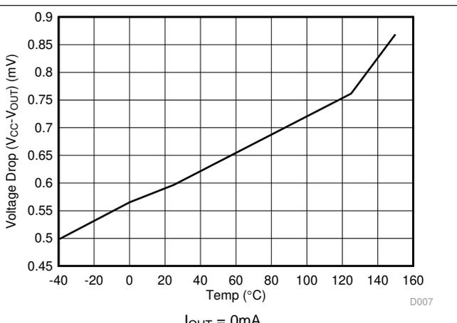
图 9. VOH (No Load) versus Temperature
