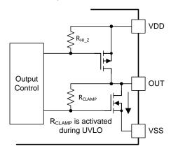
图 34. Simplified Representation of Active Pull Down Feature
