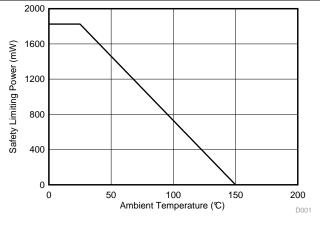
图 2. Thermal Derating Curve for Limiting Power Per VDE
