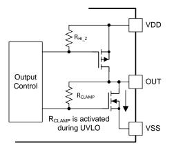
Figure 31. Simplified Representation of Active Pull Down Feature
