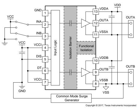
Figure 30. Simplified CMTI Testing Setup
