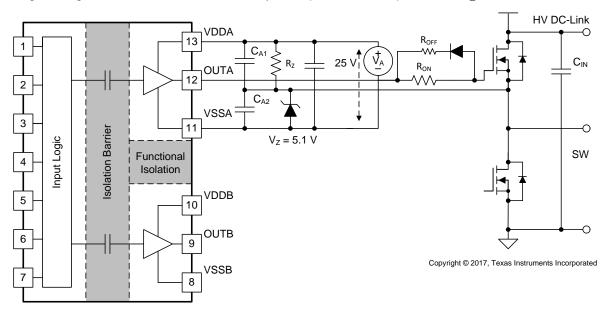
Figure 36. Negative Bias with Zener Diode on Iso-Bias Power Supply Output
