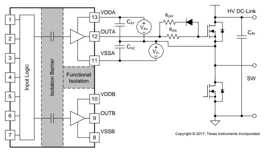
Figure 37. Negative Bias with Two Iso-Bias Power Supplies
