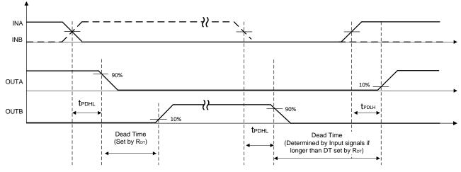
Figure 27. Dead-Time Switching Parameters
