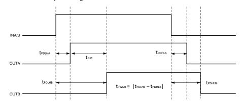
Figure 24. Overlapping Inputs, Dead Time Disabled
