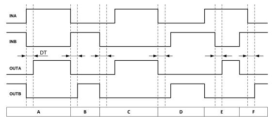
Figure 34. Input and Output Logic Relationship With Input Signals
