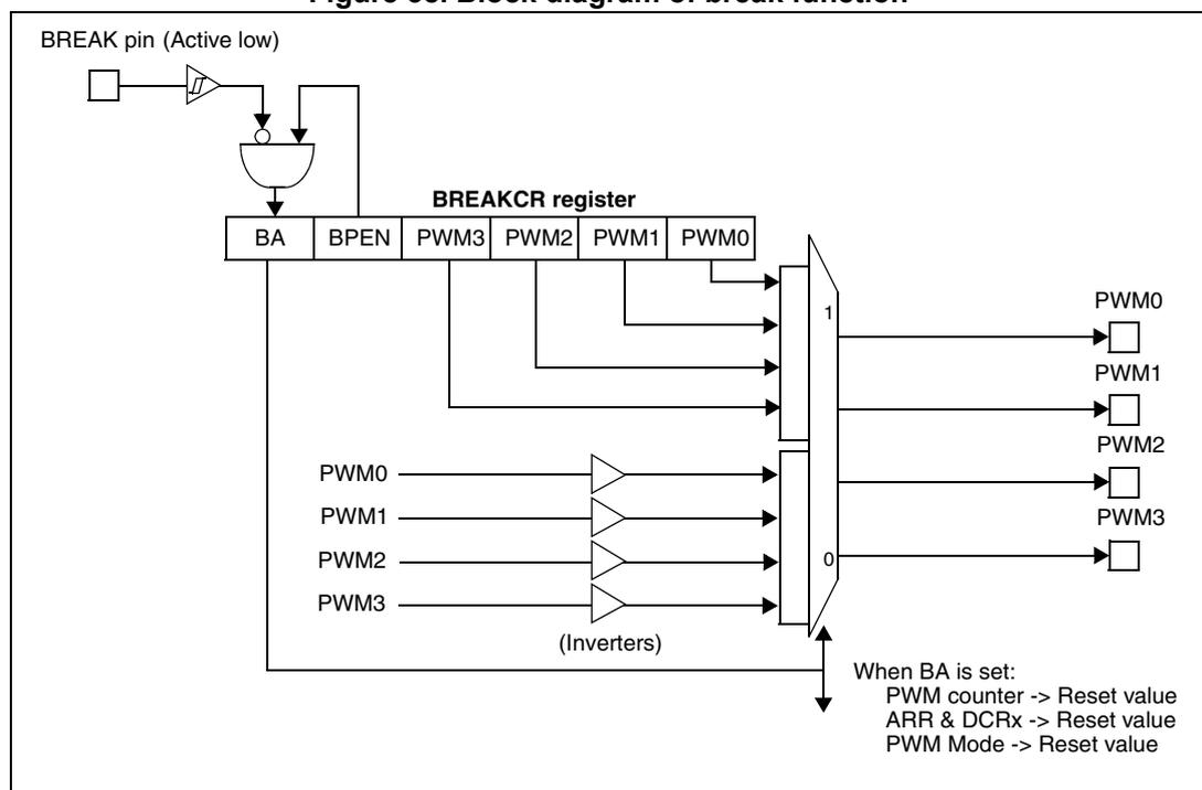
*Note:* The BREAK pin value is latched by the BA bit.
