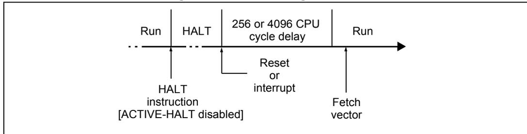
Figure 25. HALT mode flowchart
