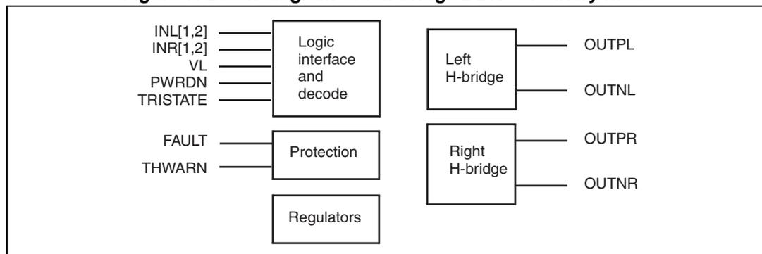
**Figure 8. Block diagram of binary half-bridge mode**
