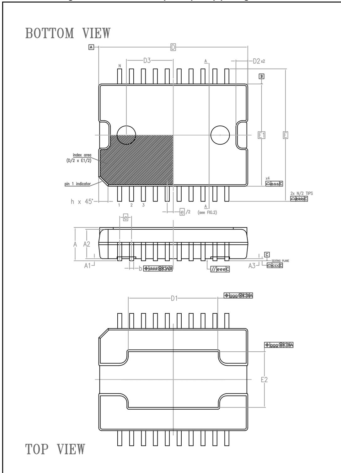
Figure 12. PowerSO-36 section A-A and B-B package outline
