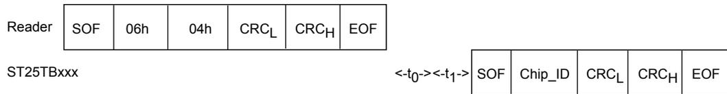
Figure 47. Slot\_marker frame exchange between reader and ST25TB512-AT
