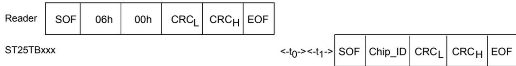
Figure 46. Pcall16 frame exchange between reader and ST25TB512-AT
