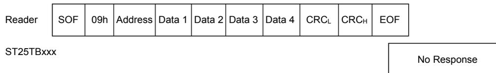
**Figure 53. Get\_UID frame exchange between reader and ST25TB512-AT**
