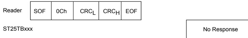
**Figure 51. Read\_block frame exchange between reader and ST25TB512-AT**
