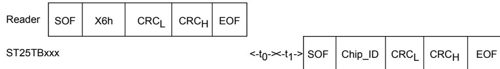
Figure 48. Select frame exchange between reader and ST25TB512-AT
