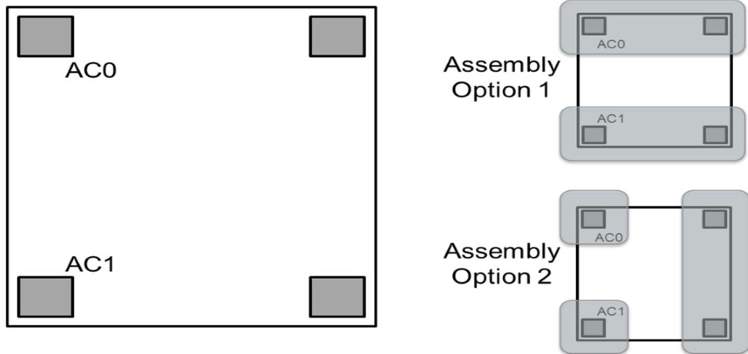
For the option 1 of the die assembly, the CTUN (referenced in [Table 13](#)) can increase from 0.5pF to 1pF. The option 2 of the die assembly is showing a tripod which can be used for physical stability, having no impact on CTUN parameter.
