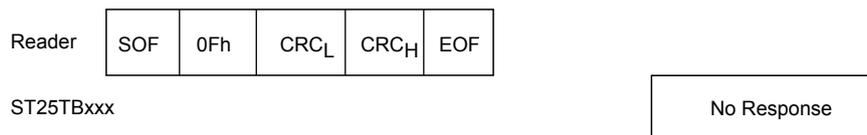
**Figure 50. Reset\_to\_inventory frame exchange between reader and ST25TB512-AT**
