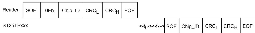
Figure 49. Completion frame exchange between reader and ST25TB512-AT
