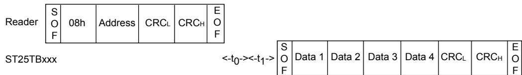
**Figure 52. Write\_block frame exchange between reader and ST25TB512-AT**
