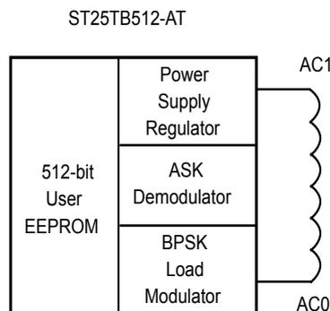
The **ST25TB512-AT** is specifically designed for short range applications that need re-usable products. The **ST25TB512-AT** includes an anticollision mechanism that allows it to detect and select tags present at the same time within range of the reader. The anticollision is based on a probabilistic scanning method using slot markers.
