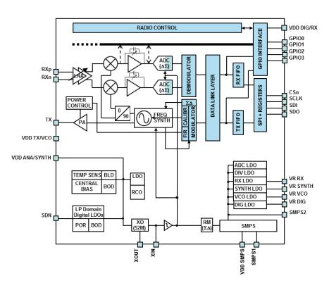
The receiver architecture is low-IF conversion, the received RF signal is amplified by a two-stage low-noise amplifier (LNA) and down-converted in quadrature (I and Q) to the intermediate frequency (IF). LNA and IF amplifiers make up the RX front-end (RXFE) and have programmable gain. At IF, the ADCs digitalize the I/Q signals. The demodulated data go to an external MCU either through the 128-byte RX FIFO, readable via SPI, or directly using a programmable GPIO pin.
