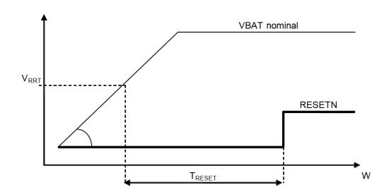
The parameters VRRT and TRESET are fixed by design in order to guarantee a reliable reset procedure of the state machine. In addition, all the registers are initialized to their default values. A software command SRES is also available, it generates an internal but partial resetting of the S2-LP.
