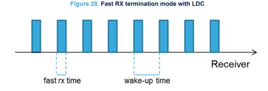
If the carrier is present, it is possible to receive the entire frame because the RX timeout stop condition is switched to the normal mechanism of PQI/SQI and SYNC can be detected:
