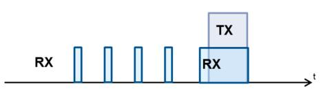
If synchronization between transmitter and receiver is required, a programmable timer value can be reloaded at SYNC word detection by the receiver or by SPI command.
