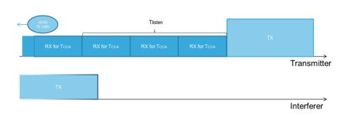
If the channel is busy and persistent\_mode bit is 0, the device will check the channel for the Tcca period. At the end, being the CS (carrier sense) signal high, it will switch in SLEEP for a randomic time that can last  $BO_{time} = T_{RCO}^* (6 + \operatorname{rand}(0: 2^{(NB+1)})^* (BU_{PRESC} + 1))$  with NB=0
