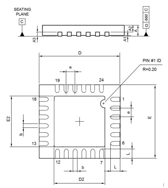
Figure 30. QFN24L (4x4 mm) package outline
