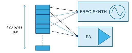
As for the normal TX operations, the TX\_FIFO samples are consumed and a management of the TX\_FIFO\_THRESHOLD is needed to perform transmissions longer than 128 samples.
