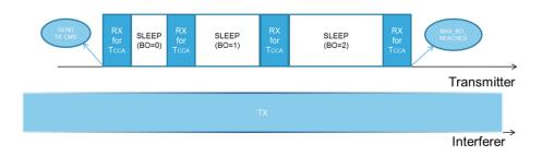
Finally, if the channel becomes free (for example during one of the SLEEP times), the device must assert channel free for a number of **NUM.\_OF\_CCA\_PERIOD** (T. listen) before transmitting:
