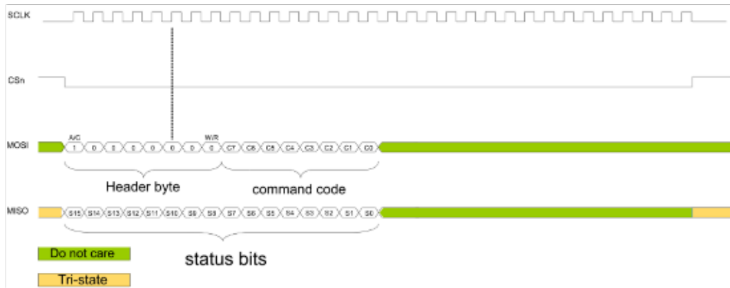
Figure 16. SPI read sequence
