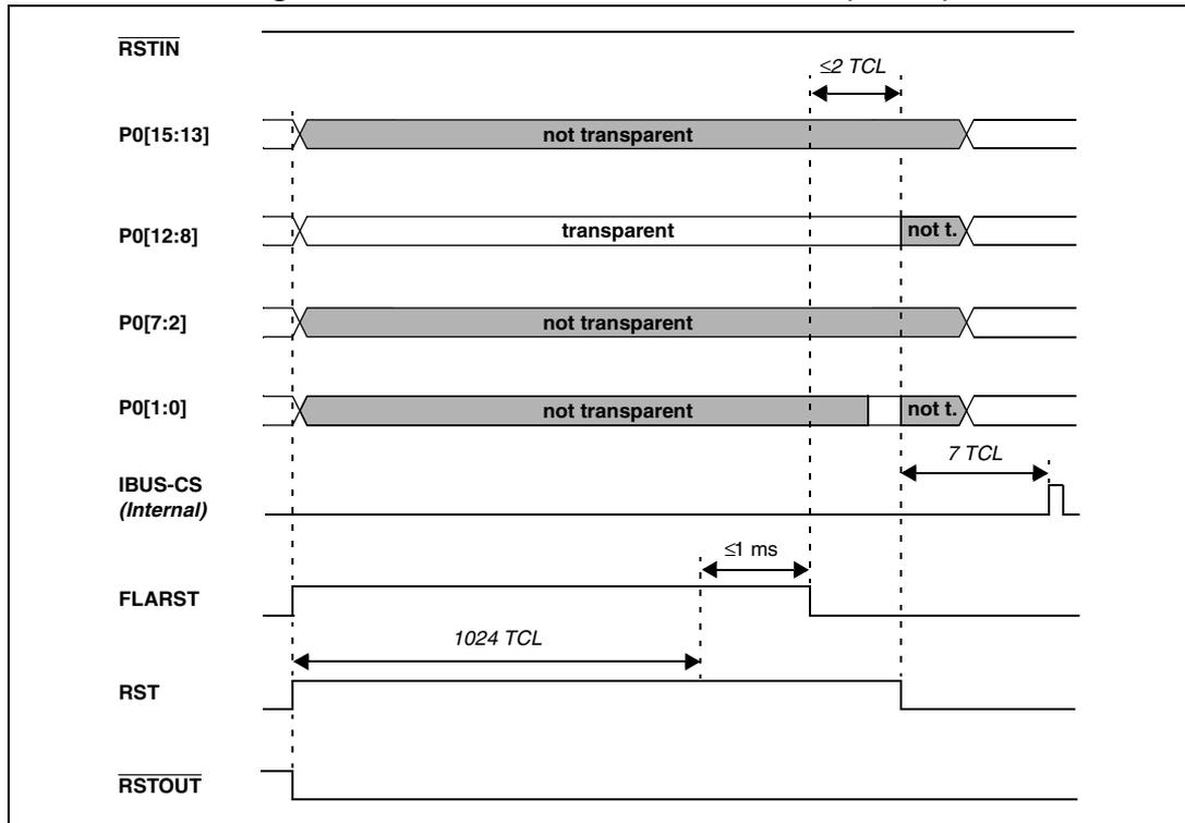
Figure 33. SW / WDT unidirectional RESET ( $\overline{EA} = 0$ )
