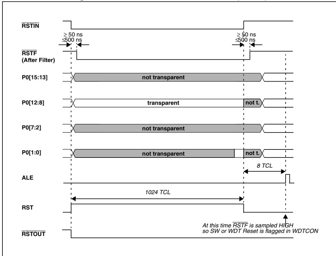
Figure 36. SW / WDT bidirectional RESET ( $\overline{EA}=0$ ) followed by a HW RESET
