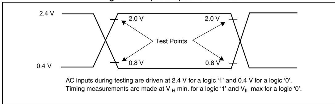
Figure 51. Float waveforms
