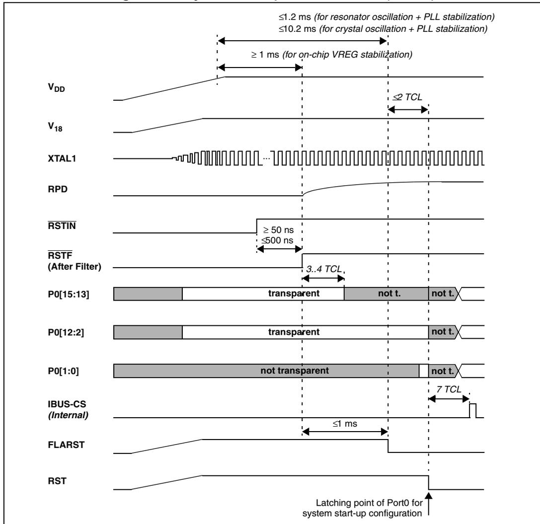
Figure 25. Asynchronous power-on RESET ( $\overline{EA} = 0$ )
