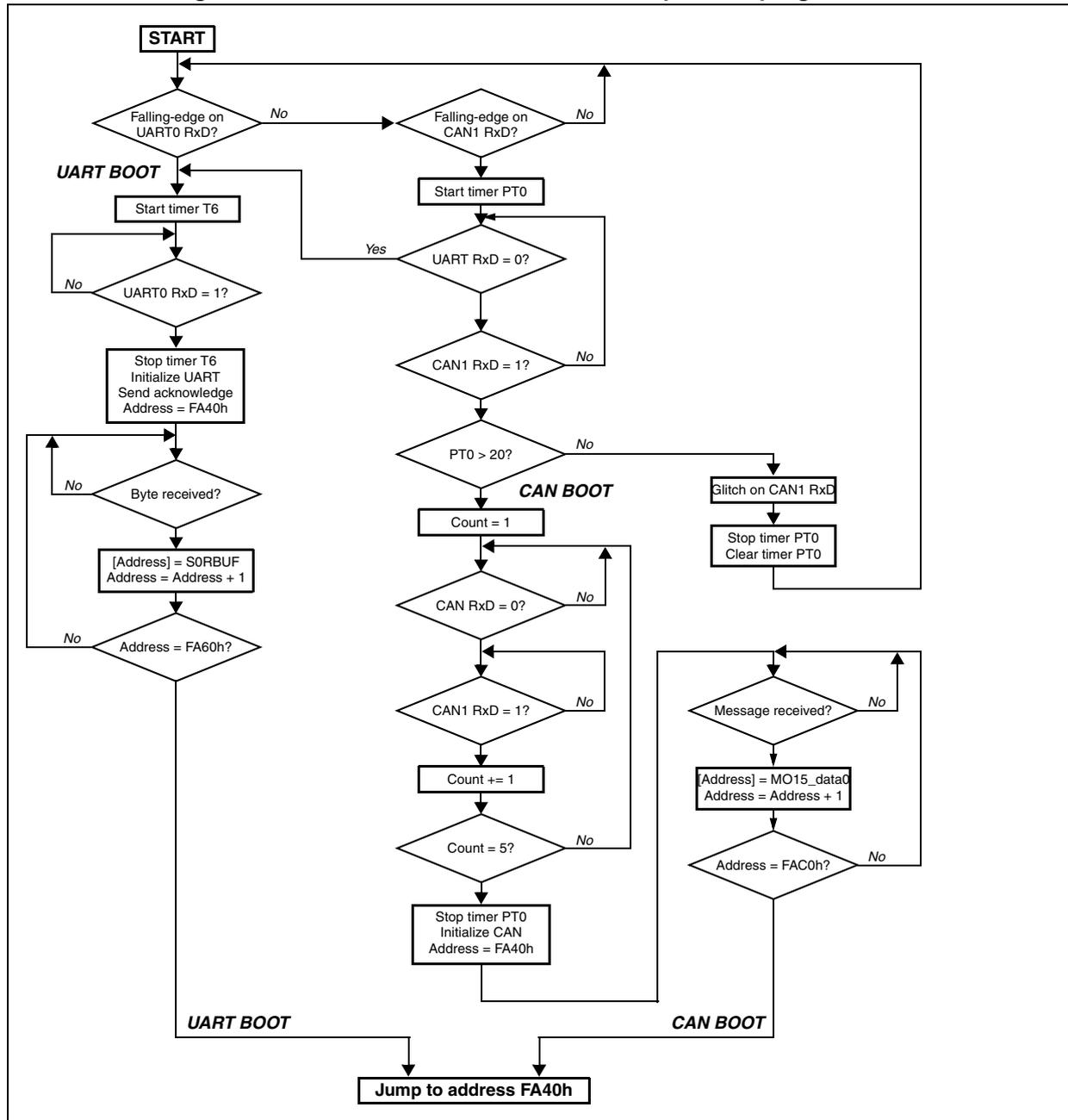
Other than after a normal reset the watchdog timer is disabled, so the bootstrap loading sequence is not time limited. Depending on the selected serial link (UART0 or CAN1), pin TxD0 or CAN1\_TxD is configured as output, so the ST10F276Z5 can return the acknowledge byte. Even if the internal IFLASH is enabled, a code cannot be executed from it.
