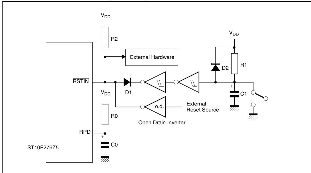
Figure 39. Internal (simplified) reset circuitry
