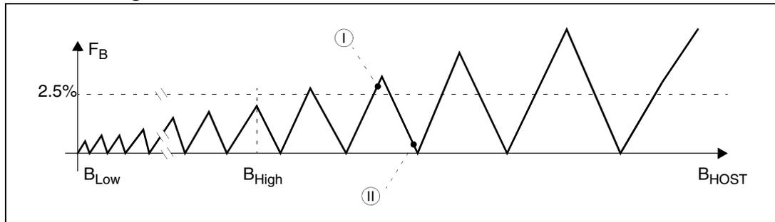
The minimum baud rate ( $B_{Low}$  in *Figure 10*) is determined by the maximum count capacity of timer T6, when measuring the zero byte, that is, it depends on the CPU clock. Using the maximum T6 count  $2^{16}$  in the formula the minimum baud rate is calculated. The lowest standard baud rate in this case would be 1200 baud. Baud rates below  $B_{Low}$  would cause T6 to overflow. In this case, ASC0 cannot be initialized properly.
