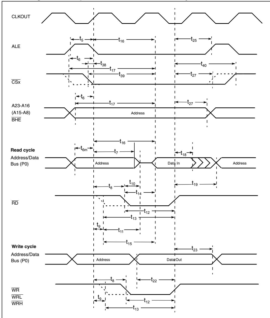
Figure 58. Multiplexed bus with/without R/W delay and extended ALE
