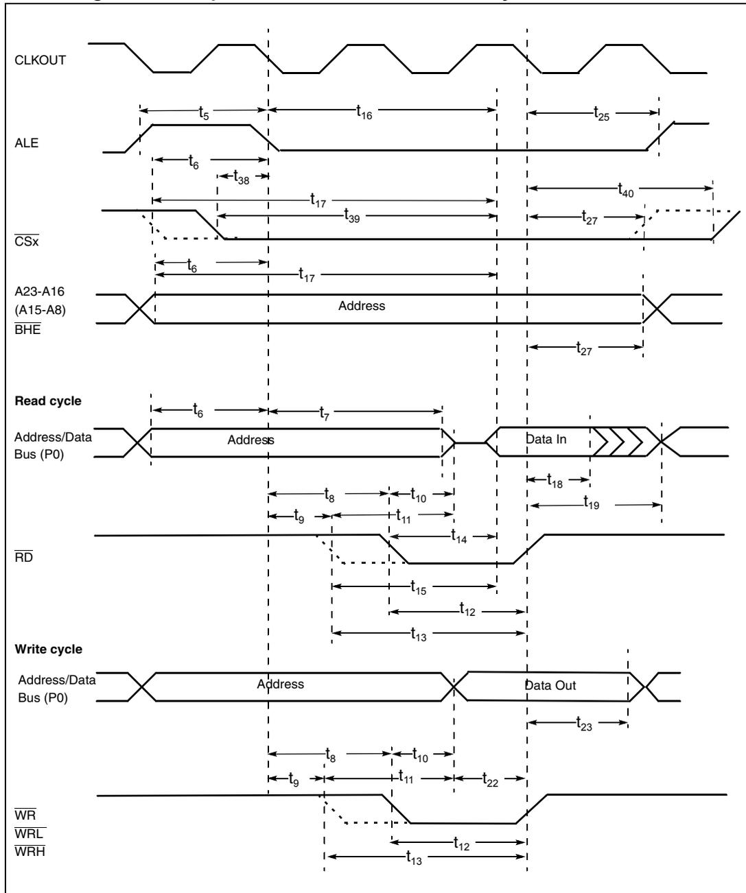
Figure 59. Multiplexed bus, with/without R/W delay, normal ALE, R/W CS
