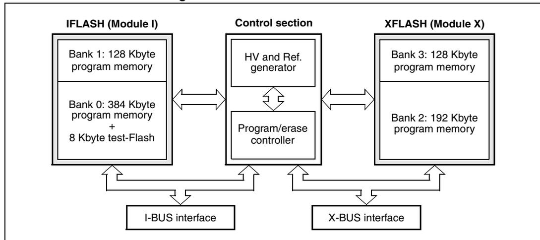
The write operations of the 4 banks are managed by an embedded Flash program/erase controller (FPEC). The high voltages needed for program/erase operations are internally generated.
