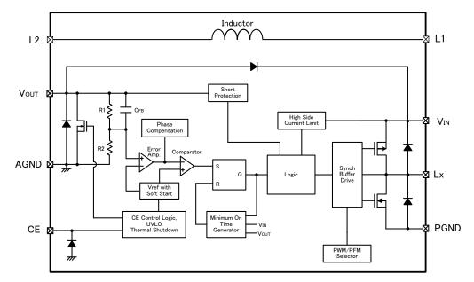
\* The XCL213 offers a fixed PWM control, a Control Logic of PWM/PFM Selector is fixed at "PWM" internally.
